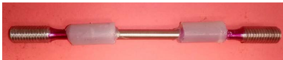
Figure 8 Detail of isolation of the zones of the specimens coincident with the wall passages of the electrolytic cell in tests according to ASTM F1624.
