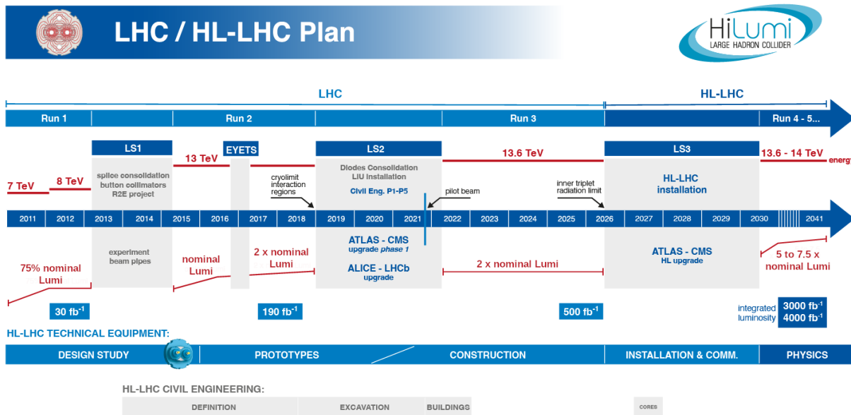
Figure 1.5: Complete LHC and HL-LHC schedule, as available at the time of writing. The collision center-of-mass energy, the peak instantaneous luminosity relative to the nominal value, and the cumulative integrated luminosity are indicated for each operation period. Image adapted from [23].
