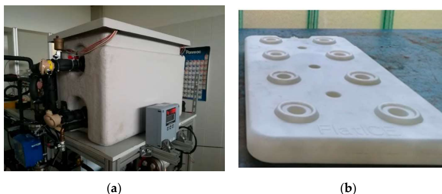
Figure 3. (a) PCM storage unit; (b) FlatICE PCM slab.
