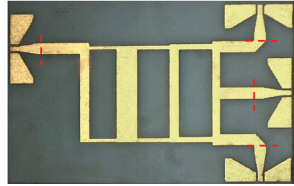
Figure 8. Prototype of 180^\circ hybrid. Reference planes for measurement and simulation are marked with red lines.
