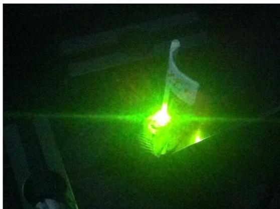
**Figure 3.19:** Up-conversion luminescence of the  $\text{Gd}_2\text{O}_3\text{:10\%Er}^{3+}$  sample upon 980 nm excitation at room temperature.
