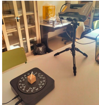
Figure 6. Fixed scanning with a rotating platform of the EinScan Pro HD scanner.
