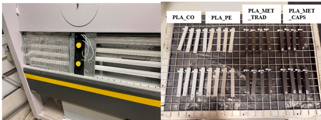
Figure 4. UV test equipment and arrangement of the test tubes on the metal grids.
