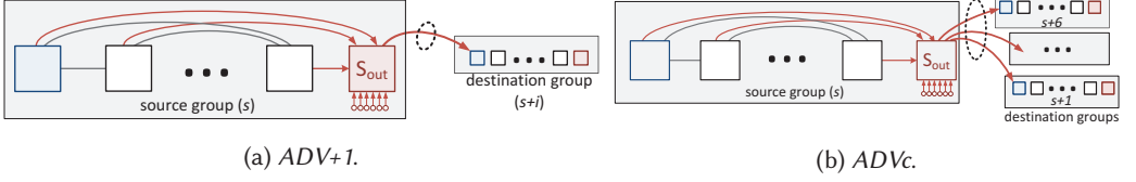
Fig. 4. ADV+i and ADVc in a Dragonfly network with h = 6 , t = 1 . On the left, traffic from each source group s goes to group s + i through t global links and on the right, it goes to the next h = 6 consecutive groups through the circled links.
