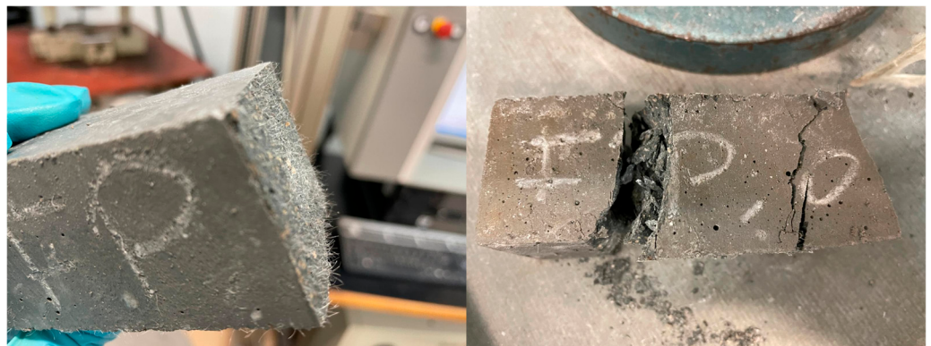
Figure 5. Prismatic samples after flexural test (left) and compression test (right). Mortars with PP fibers.
