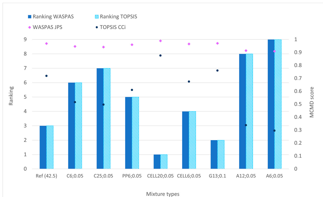
Figure 12. MCDMA results: mortars with fibers (excluding the “printability index” criteria).
