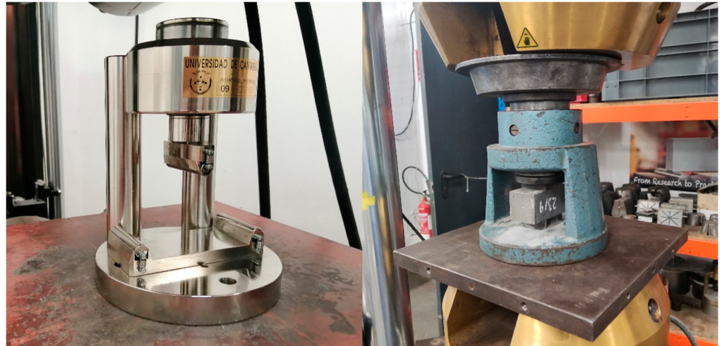
Figure 4. Flexural test (left); compression test (right).
