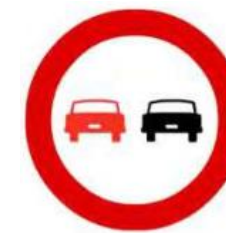
Figure 10: TR-305 signal, overtaking prohibition.
