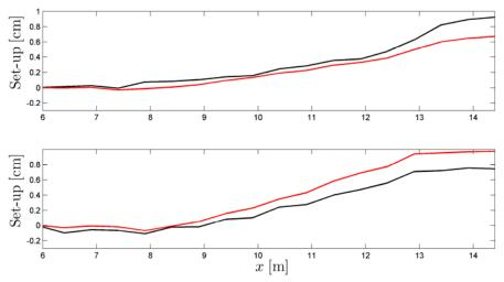
Figure 7. Cross-shore evolution of mean water level. Upper panel: rip channel; lower panel: rip-trough. Black line: observed; red line: calculated from radiation stress gradient (equation 7).
