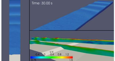
Figure 5. Snapshot of regular waves interacting with a bar and a narrow cross-shore channel. Left panel: top view of the free surface. Upper panel: side view of the free surface. Lower panel: cross shore transects of horizontal velocity.
