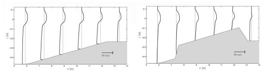
Figure 8. Cross-shore transect of mean currents. Left panel: rip channel; right panel: rip-trough.
