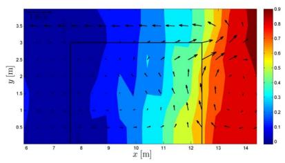
Figure 6. Mean surface elevation (set-up) in cm. Black arrows indicate depth-averaged mean currents. Waves are propagating from left to right.
