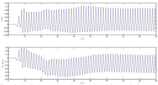
Figure 2: Evolution of the free surface (top panel) and cross-shore velocity (bottom panel) at 1/3 of the water depth from the bottom, within the rip channel (X = 10 m, Y = 3.5 m).
