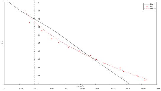
Figure 3: Cross-shore velocity as function of long-shore positions at x = 11.40 m, at 1/3 of the depth from the bed.
