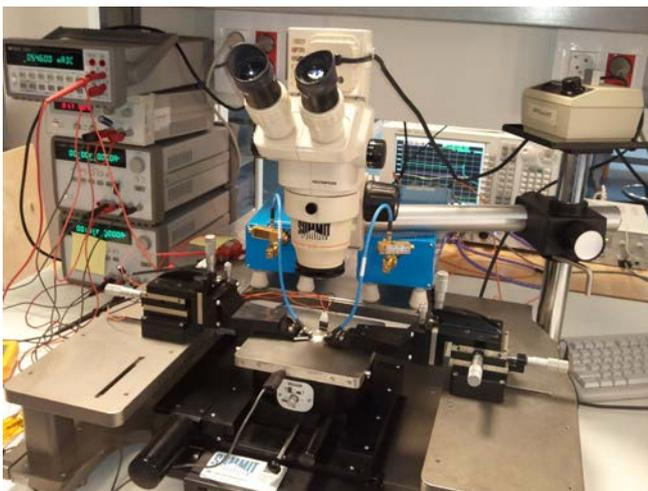
Fig. 34. Laboratory set-up for on wafer measurements of MMICs
