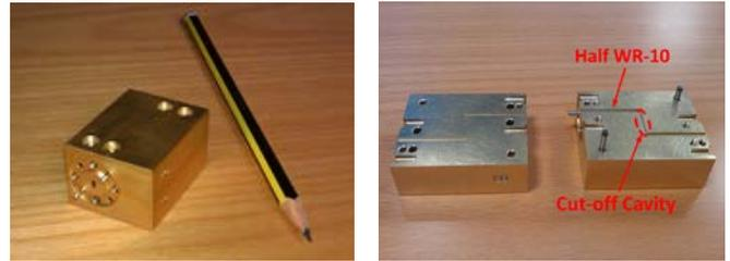
Fig. 44. Photographs of the Metal Case for the Back-to-Back Transition ( $4 \times 3 \times 2.4 \text{ cm}^3$ )
