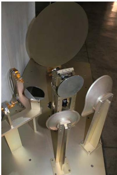
Fig. 14. 300GHz antenna prototype
