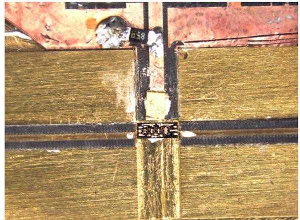
Fig. 54. Amplifier MMIC placed on the box. Both finline transitions as well as the DC biasing are connected by wire bonding
