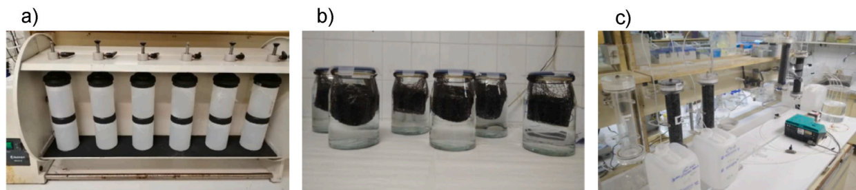
Fig. 1. Images of the experimental developments of the leaching tests: a) Compliance leaching test (EN 12457) or pH-dependency leaching test (EN 14429), b) Dynamic Surface Leaching Test (DSLTL, CEN/TS 16637-2) and c) Up-flow percolation leaching test (CEN/TS 16637-3).
