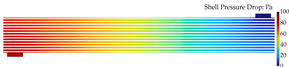
Fig. 11. Pressure drop profile in the shell compartment for [emim][Ac] using the PS HFMC.
