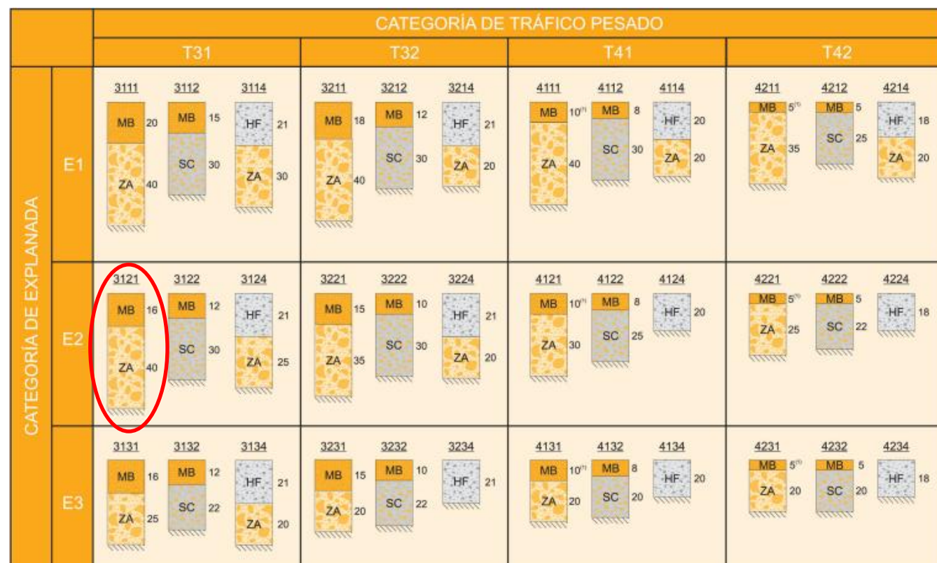
Figure 3. Catalogue of Pavement Sections for Heavy Traffic Categories T31 to T42.
