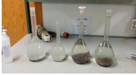
Figure 10. Determination of the mass of the displaced water.
