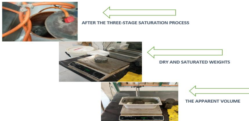
Figure 12. Illustration of the procedure applied to determine the physical properties of the composites (specimen).
