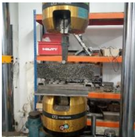
Figure 15. Setup demonstrating a specimen subjected to the flexural test.
