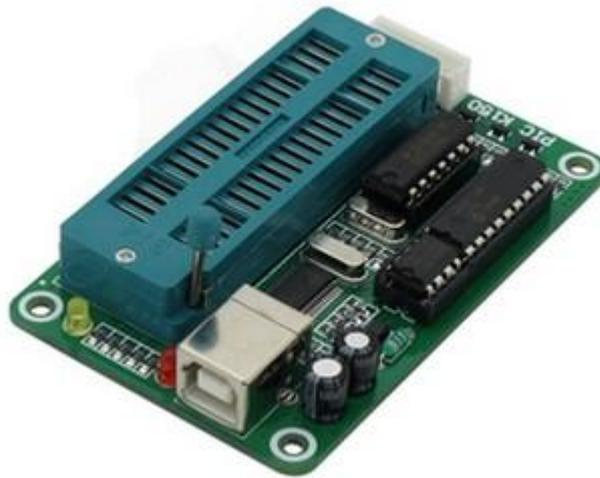
Figura 72 Tarjeta programadora K150.
