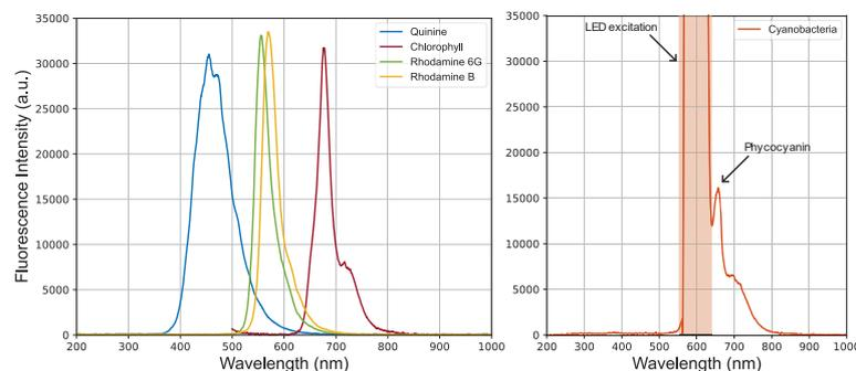
Figure 2. Fluorescence spectra obtained of quinine, rhodamine 6G, rhodamine B, chlorophyll, and phycocyanin in a cyanobacteria culture, excited with 373 nm, 520 nm, 520 nm, 451 nm, and 615 nm LEDs, respectively. The saturated region in the cyanobacteria spectrum corresponds to scattered LED light, while the adjacent peak represents phycocyanin fluorescence.
