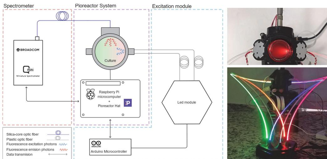
Figure 1. Configuration of the fluorescence sensor integrated into the photobioreactor. On the left, a simplified diagram illustrates the overall configuration. The top-right image shows the reactor vial open from the top, providing an example of how the optical fiber excites the sample. The bottom-right image depicts the LED module, which couples the light into the plastic optical fibers to guide it toward the sample.
