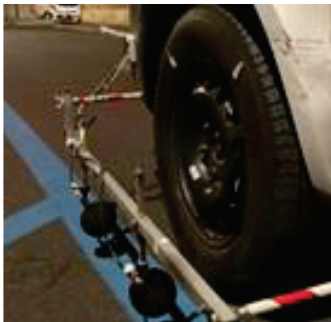
Figure 3: Schematic representation of the CPX measurement system
