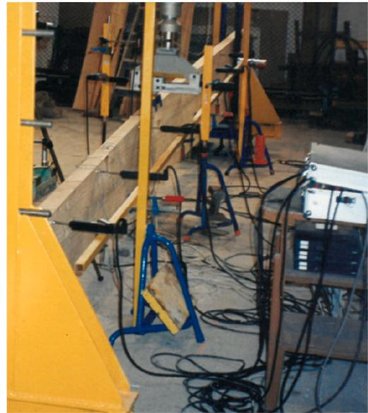
Fig. 7. Horizontal transducers to estimate the shape of the initial imperfection of the beams.
