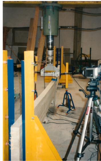
b. Lateral buckling deformation II.
