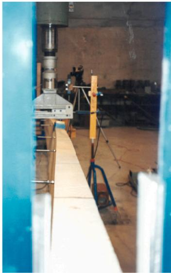
a. Lateral buckling deformation I.
