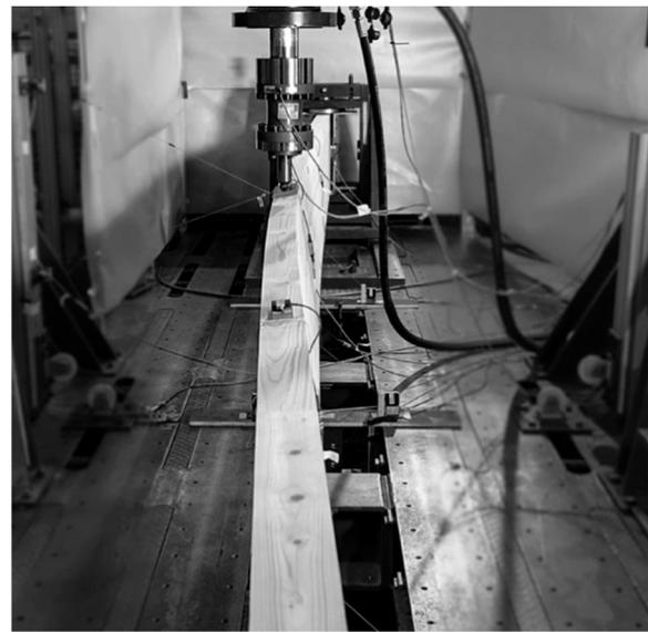
Fig. 6. Wilden, Hoffmeister & Feldmann test on glued laminated timber [12].
