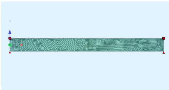
a. Elevation view of the constant depth beam N°2 without deforming (plate type model).
