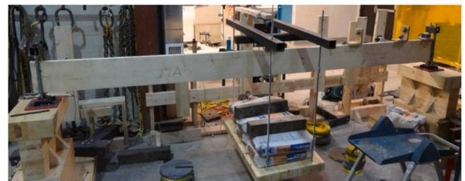
Fig. 3. Xiao test on lumber joists (glued laminated timber) [7].
