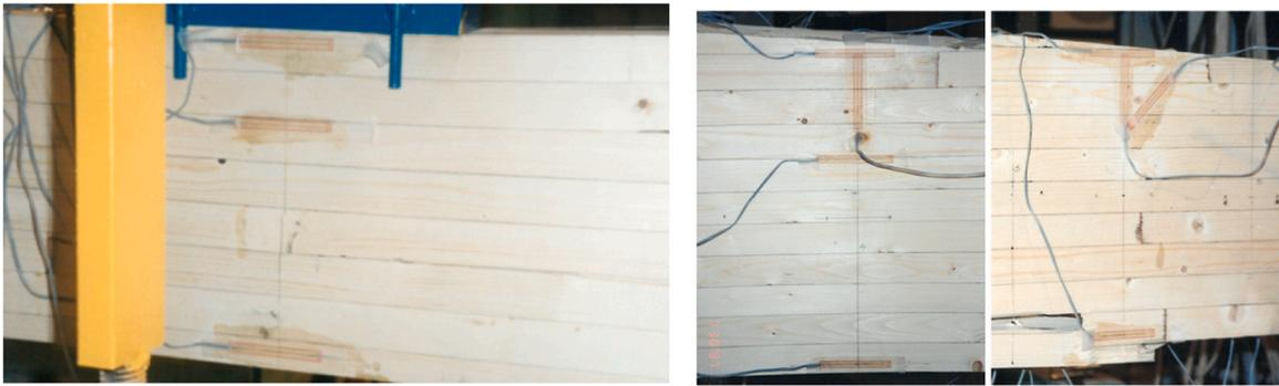
a. Extensometric bands on a constant depth beam.
