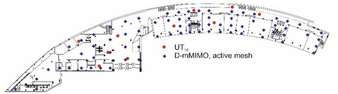
Figure 4. Optimized D-mMIMO mesh topology for UT<sub>10</sub> (73 antennas).
