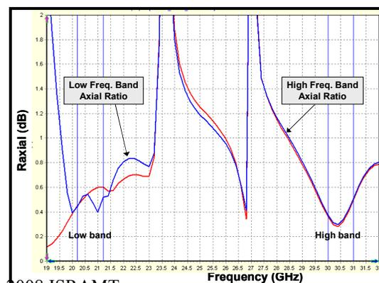
Fig.8. Axial Ratio of the septum polarizer
