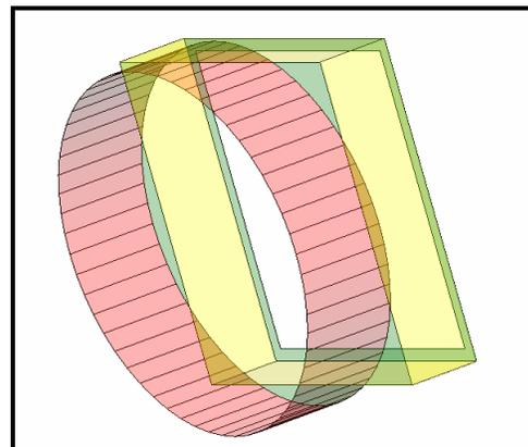
Fig.6. Squared - circular waveguide transition for the common port
