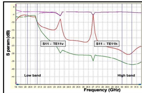
Fig.8. Polarizer performance at the circular ports
