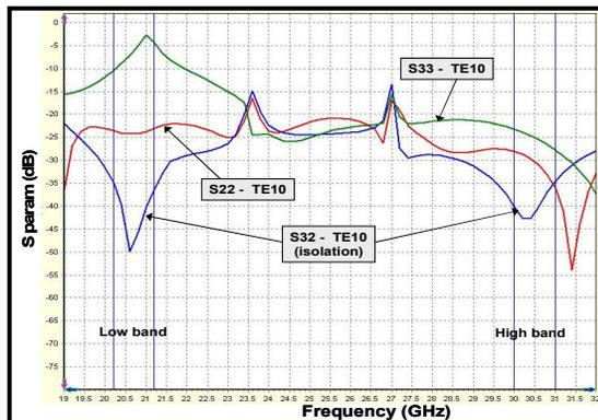
Fig.7. Polarizer performance at the rectangular ports
