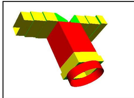
Fig.1. 3D model of the dual-band septum OMT Polarizer
