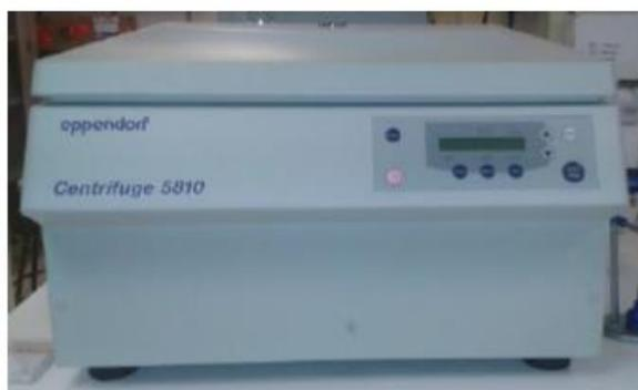
**Figura 2.5 Centrífuga Eppendorf 5810.**
