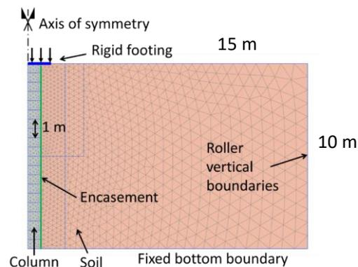
Figure 2. Numerical model and finite element mesh.
