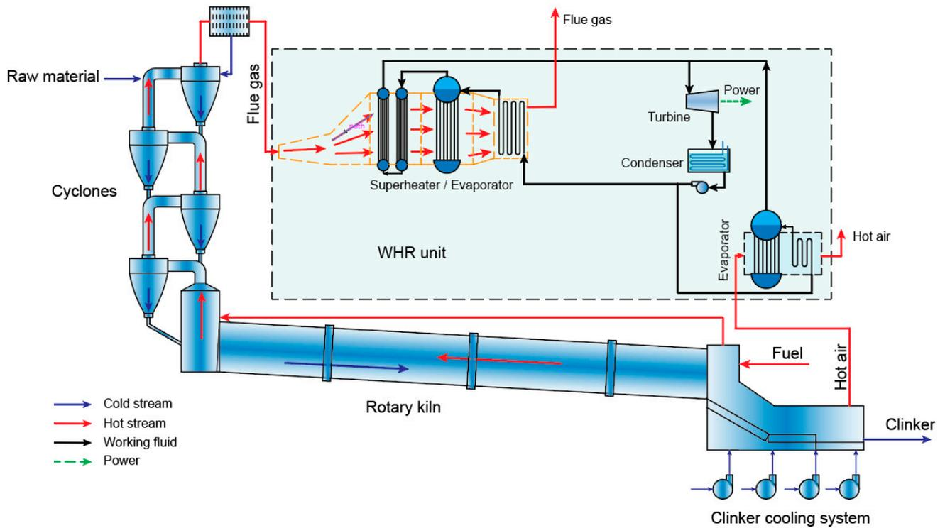
**Figure 1.** Schematic of a WHR system in cement production (source: own elaboration).
