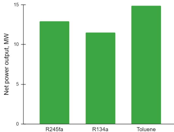
**Figure 2.** Net power output values of the WHR using different working fluids.
