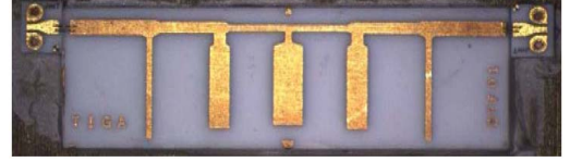
Fig. 6. Designed band pass filter together with coplanar-microstrip transitions.
