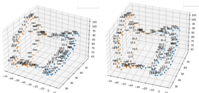
Fig. 5. In the first run the lines confuse the algorithm, in the second run with other initial points within the crowns (randomly chosen) it is able to ignore them, the nan values appear on the lines and not on the crowns.
