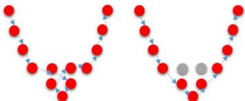
Fig. 6. On the left the wrong loop sequence is generated (although the image is in 2D, 3D is required in order to happen). On the right the expected sequence with two lesions in gray ignored.
