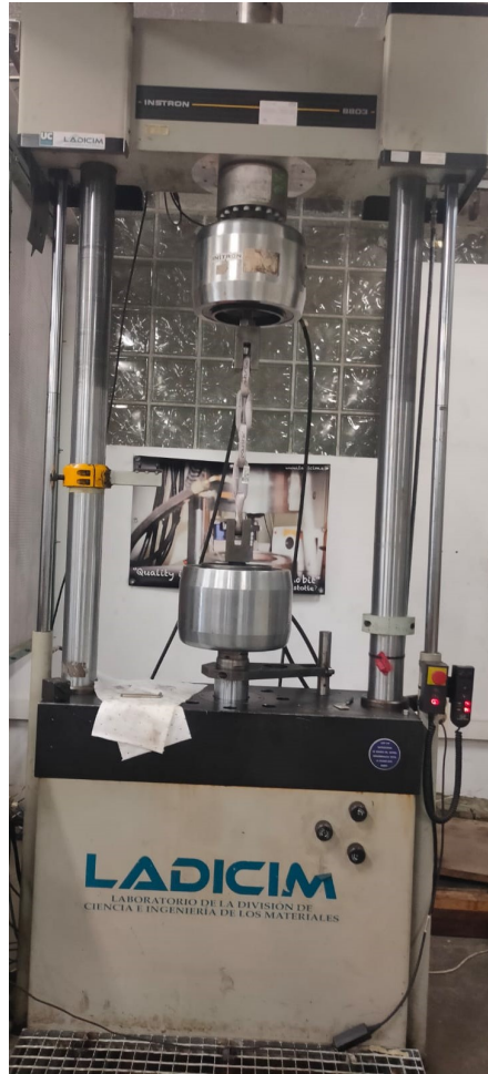
Figure 10: Experimental set up with the Dyneema chain sample secured at both ends, with a total of five links.
