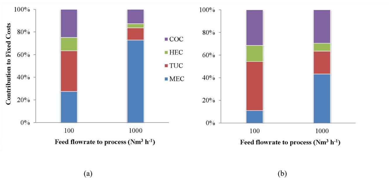
**Figure 4.** Contribution of terms (in percentage values) to fixed costs (FC): membrane units (MEC), turbine (TUC), heat exchangers (HEC), compressors (COC). Plant capacities of 100 and 1000 ( $\text{Nm}^3 \text{h}^{-1}$ ) feed flowrate basis, operating at two pressure ratios (a) 4:0.5, (b) 8:0.5, bar basis.
