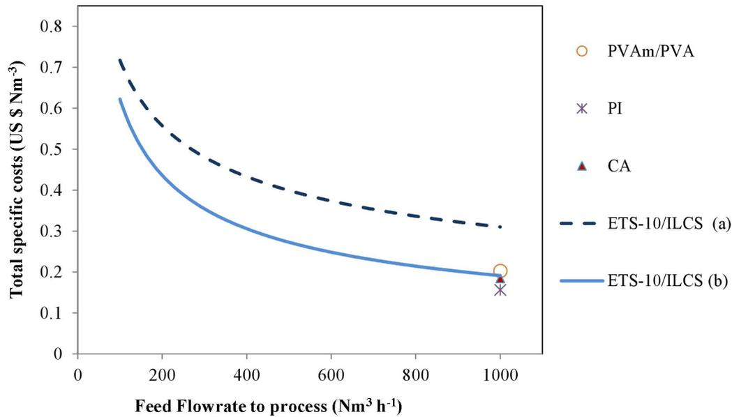
**Figure 2.** Trend of total specific costs per unit plant capacity, from 100 to 1000 Nm<sup>3</sup> h<sup>-1</sup>. Comparison for the two operating pressure ratios (a) 4:0.5 (b) 8:0.5, bar basis, using the ETS-10/ILCS membrane. References of other reported membranes, 1000 Nm<sup>3</sup> h<sup>-1</sup> feed flowrate basis: PVAm/PVA blend <sup>20</sup>, PI and CA <sup>22,24</sup>
