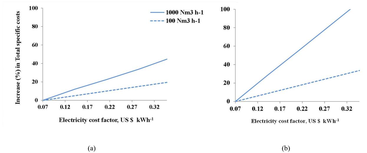
**Figure 7.** Increase (%) in Total specific costs of the separation process versus cost of electricity (a) (*Zelec*, US\$ kWh<sup>-1</sup>). Plant capacities of 100 and 1000 (Nm<sup>3</sup> h<sup>-1</sup>) feed flowrate basis, operating at two pressure ratios (a) 4:0.5, (b) 8:0.5, bar basis.
