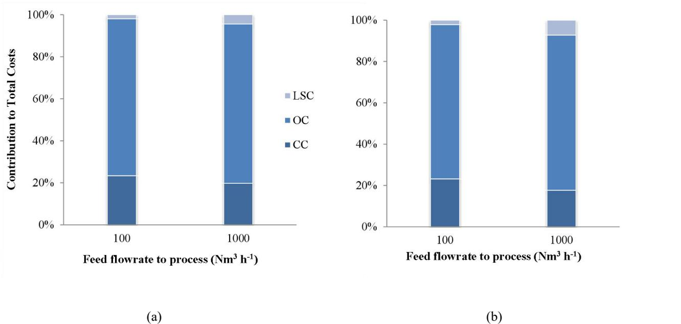
**Figure 3.** Contribution of terms in total costs (TC): capital costs (CC), operating costs (OC), and cost of losses for CH<sub>4</sub> (LSC). Plant capacities of 100 and 1000 (Nm<sup>3</sup> h<sup>-1</sup>) feed flowrate basis, operating at two pressure ratios (a) 4:0.5 (b) 8:0.5, bar basis.
