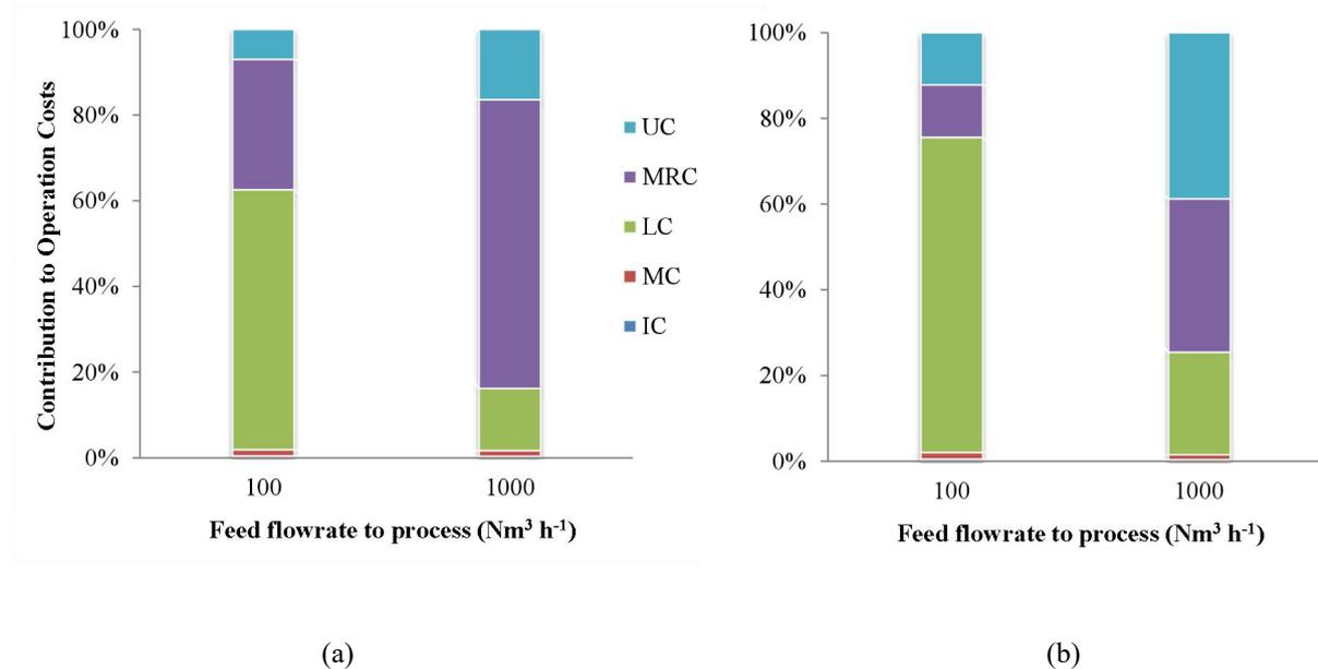
**Figure 5.** Contribution of terms (in percentage values) to operational costs (OC): utilities (UC), membrane replacement (MRC), and labour (LC); maintenance (MC) and insurance costs (IC). Plant capacities of 100 and 1000 ( $\text{Nm}^3 \text{h}^{-1}$ ) feed flowrate basis, operating at two pressure ratios (a) 4:0.5, (b) 8:0.5, bar basis.
