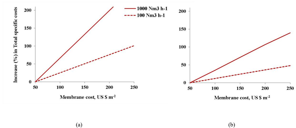
**Figure 6.** Increase (%) in total specific costs of the separation process versus cost of membrane ( $Z_{mem}$ , US\$ m<sup>-2</sup>). Plant capacities of 100 and 1000 (Nm<sup>3</sup> h<sup>-1</sup>) feed flowrate basis, operating at two pressure ratios (a) 4:0.5, (b) 8:0.5, bar basis.
