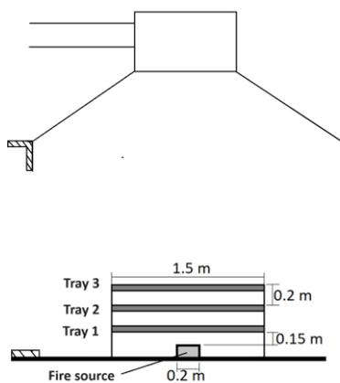
**Figure 1.** Front view of the test set-up.
