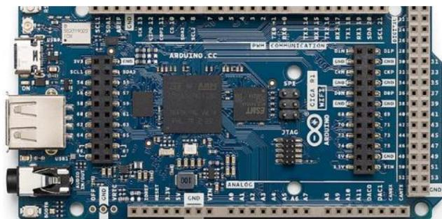
Figura 3. Arduino Giga R1
