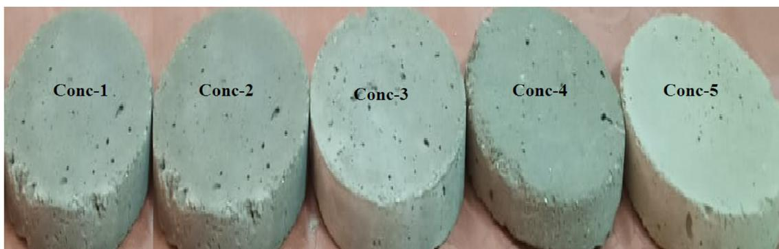
Fig. 1 – Part of prepared samples for radiation shielding measurements with thickness 3 cm.
