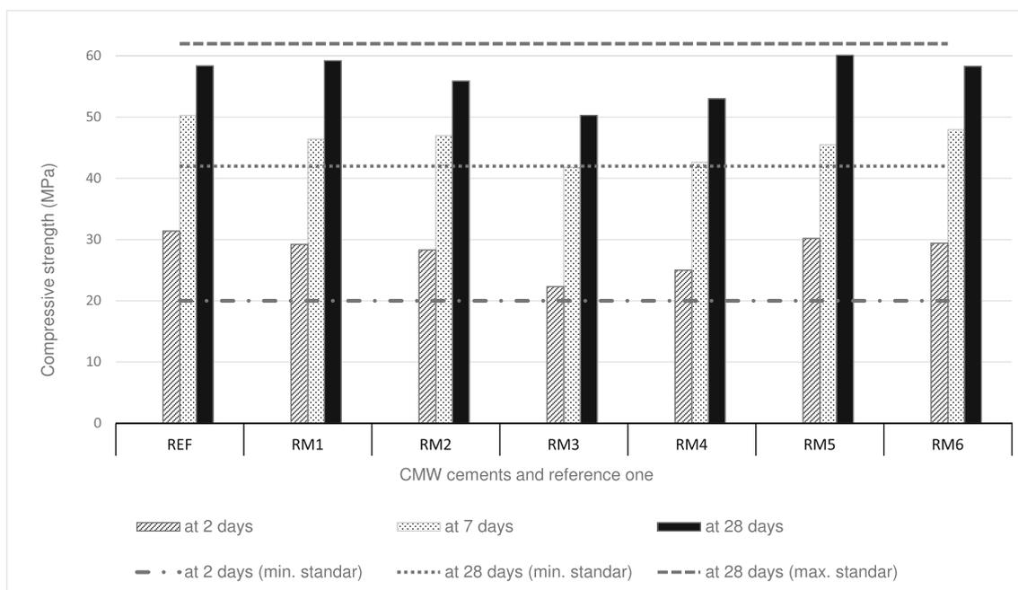
Fig. 5 Compressive strength results at the ages of 2, 7, and 28 days
