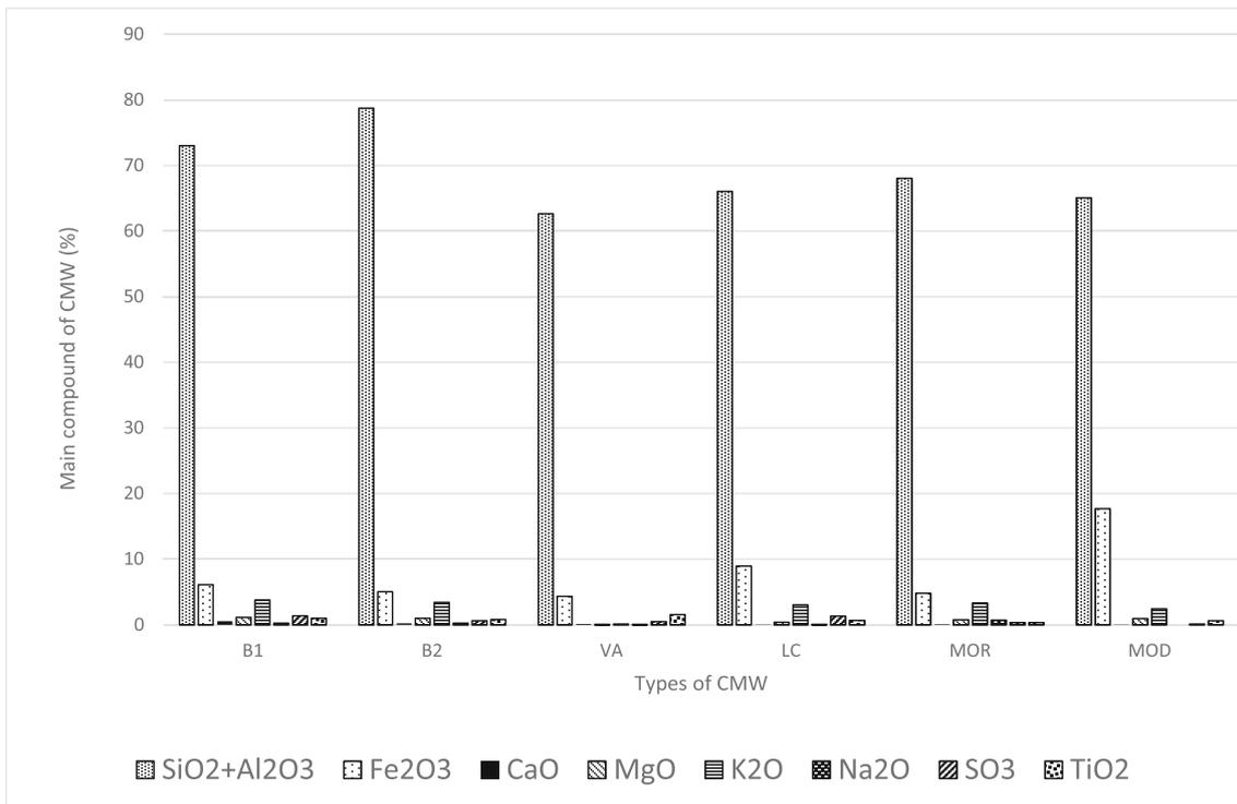
Fig. 3 Main compound of CMW, highlighting the SiO<sub>2</sub> and Al<sub>2</sub>O<sub>3</sub>
