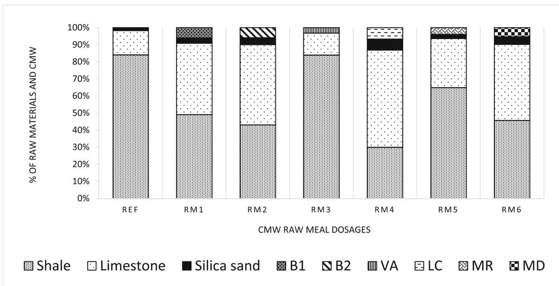
Fig. 4 raw meal dosages of the reference clinker and calculated CMW clinker
