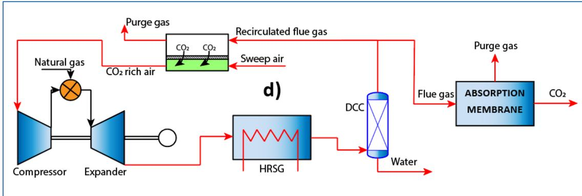
Figure 5.6. CO<sub>2</sub> capture with SEGR – MEA absorption (case 7) and membrane separation (case 8).
