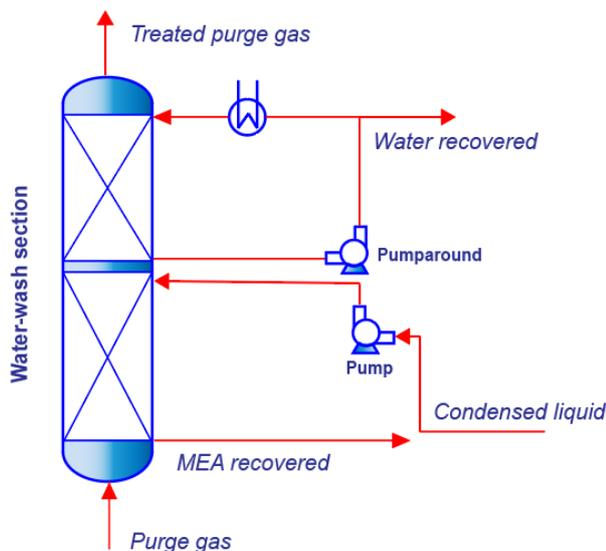
Figure 4.4. Water-wash section flowsheet of the absorber column.
