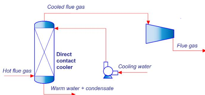
Figure 4.1. Flue gas pre-treatment unit.
