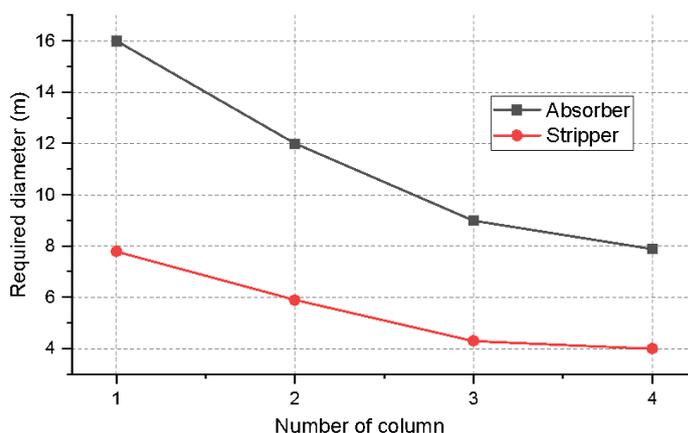
Figure 4.3. Absorber/stripper diameter versus the number of column.
