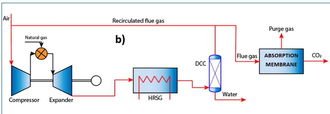
Figure 5.4. CO<sub>2</sub> capture with EGR – MEA absorption (case 3) and membrane separation (case 4).
