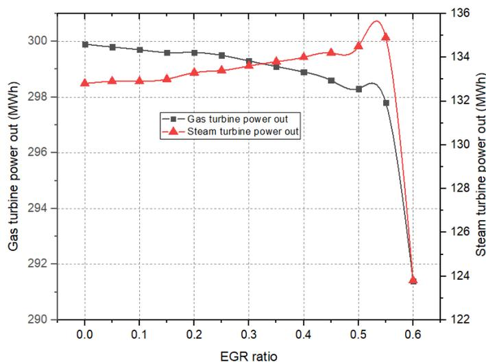
Figure 3.6. The effect of exhaust gas recirculation on the power output of the gas turbine and steam turbines.
