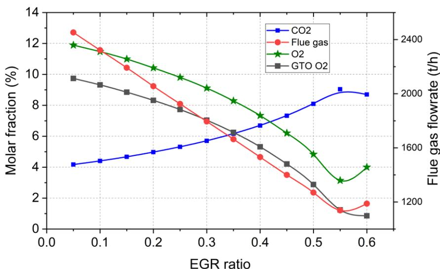
Figure 3.5. The effect of exhaust gas recirculation in different ratios on the exiting flue gas mass flowrate and the molar concentration of different compounds.
