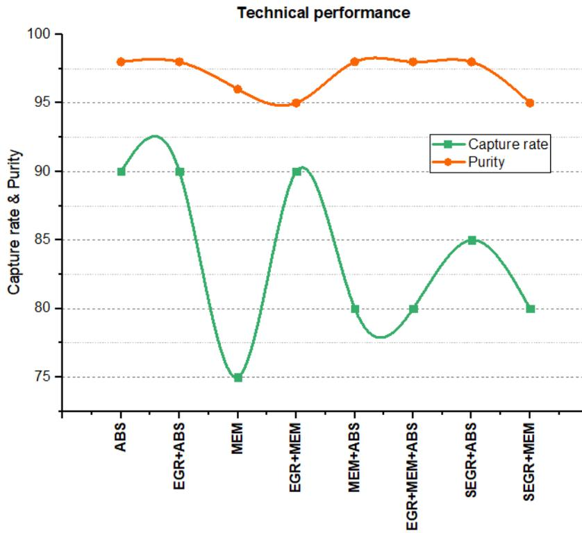
Figure 5.7. The technical performance of various carbon capture technologies, focusing on two key metrics: CO<sub>2</sub> capture rate and CO<sub>2</sub> purity.
