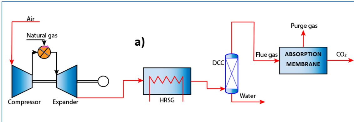
Figure 5.3. CO<sub>2</sub> capture non-EGR/SEGR – (baseline) MEA absorption (case 1) and standalone membrane separation (case 2).
