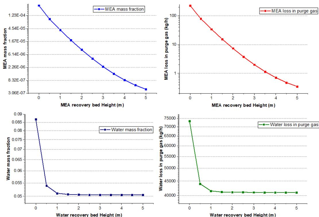
Figure 4.5. Effect of water-wash section packing height on MEA and water reduction in purge gas.
