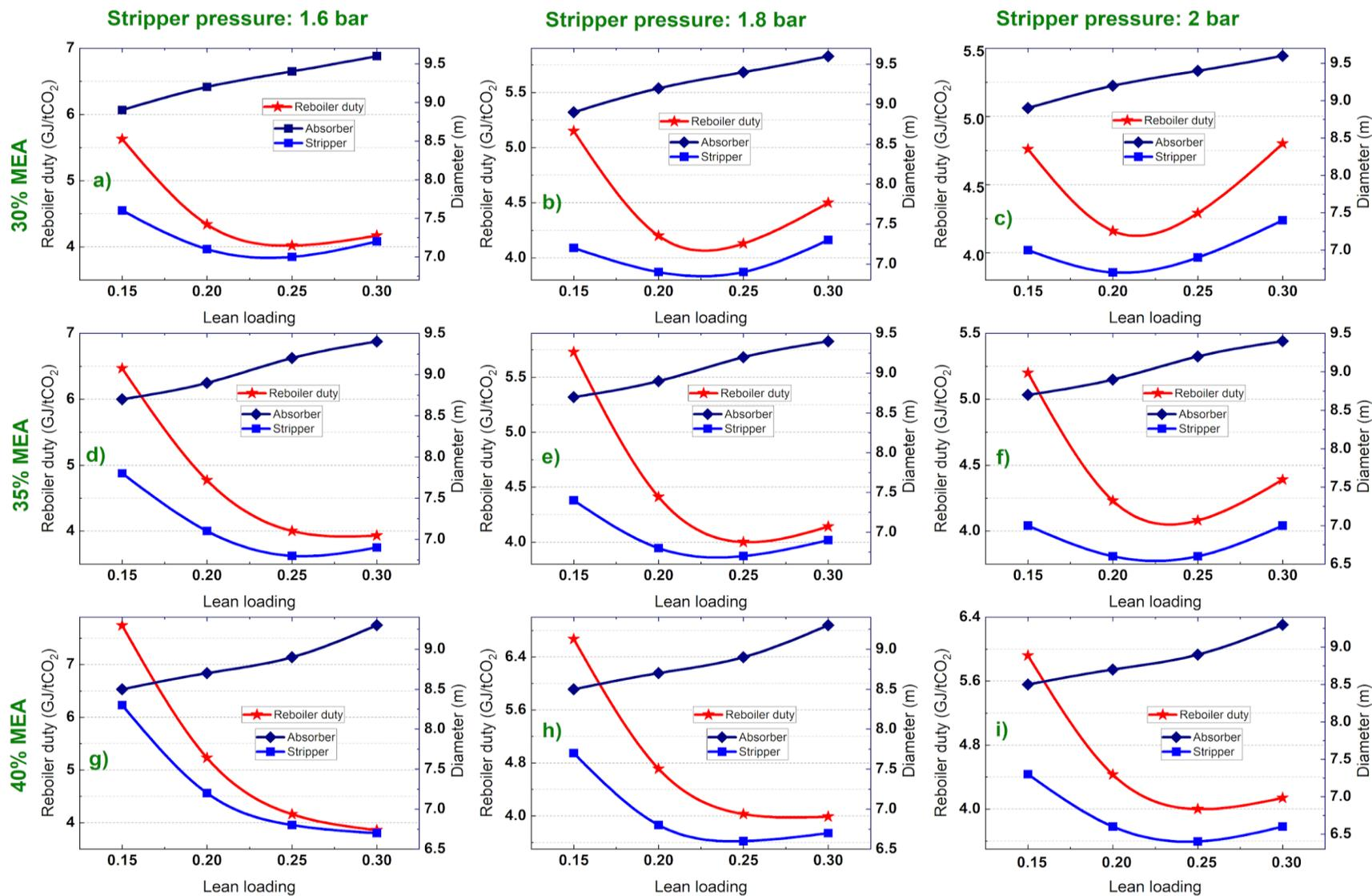
Figure 4.9. Relationship between lean amine loading, reboiler duty, and column diameter (absorber and stripper) for various MEA concentrations (30%, 35%, 40%) at stripper pressures of 1.6, 1.8, and 2 bar. Each subplot (a–i) represents a specific combination of these conditions.
