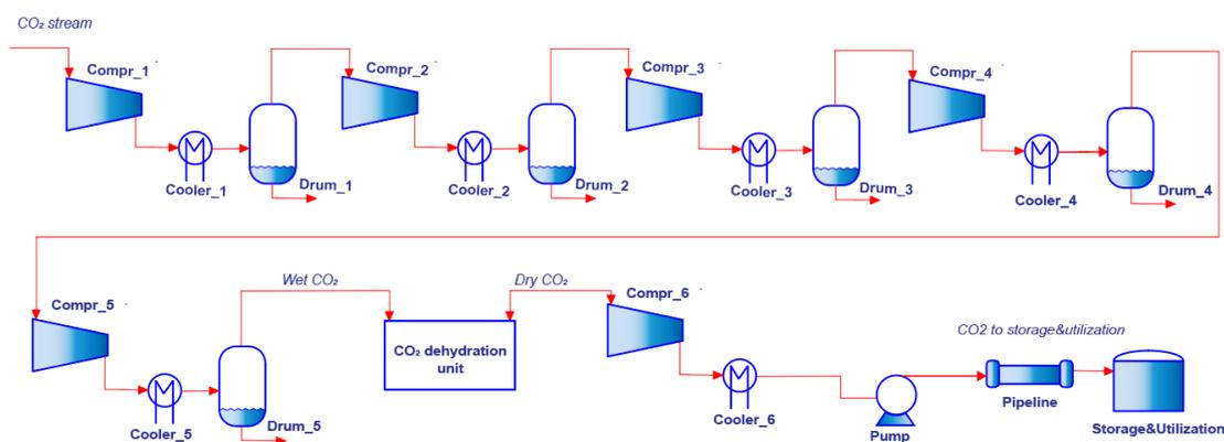
Figure 4.6. The flowsheet of CO<sub>2</sub> dehydration, compression, and pipeline transportation to the enhanced oil recovery storage site.
