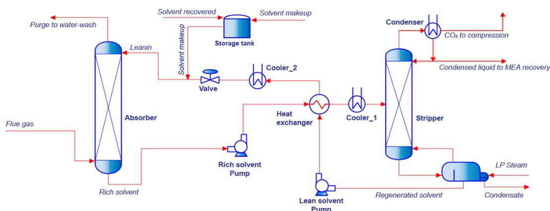
Figure 4.2. The general flowsheet of the MEA absorption-based PCC plant.
