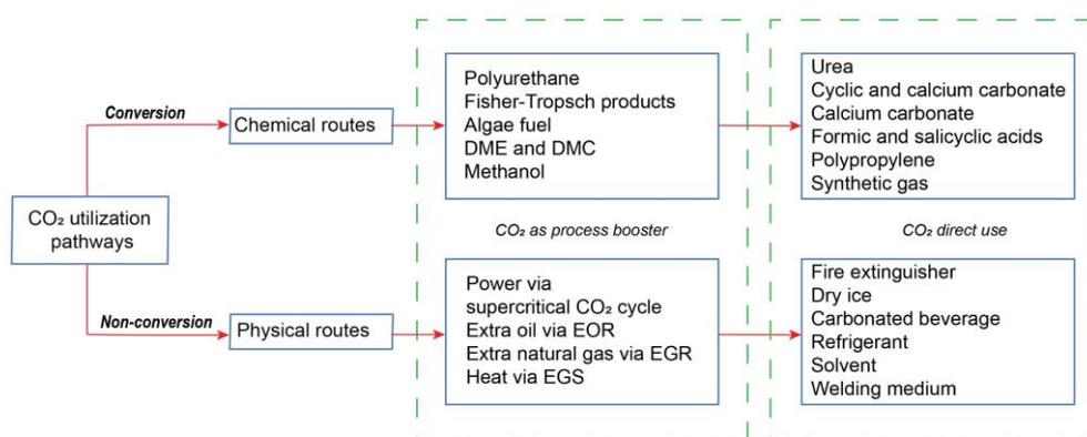
Figure 1.3. CO<sub>2</sub> utilization pathways by categories (Based on [34]).
