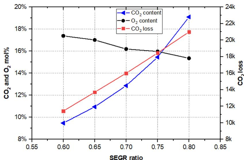
Figure 5.1. The effect of SEGR in different ratios on CO<sub>2</sub> molar fraction in the flue gas leaving the HRSG to PCC, O<sub>2</sub> molar fraction before the combustion chamber, and CO<sub>2</sub> loss in SEGR unit.
