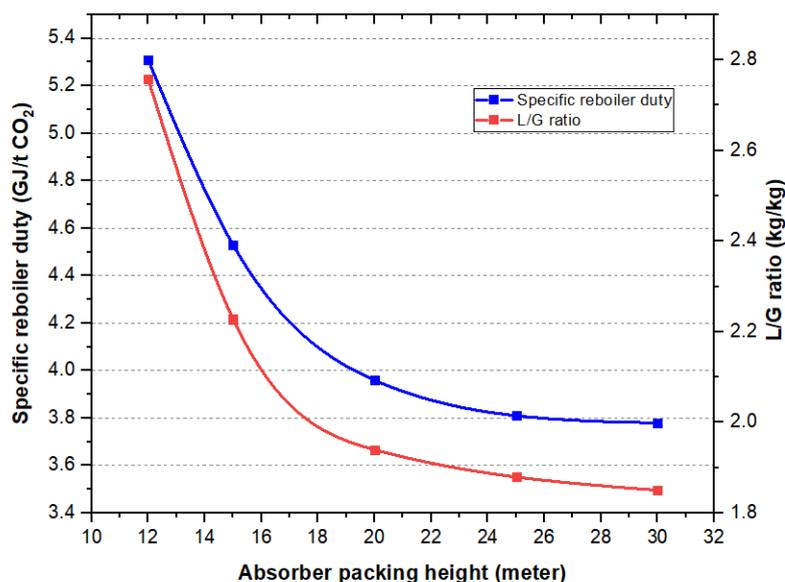
Figure 4.10. Relationships between the absorber packing height and specific booster duty and L/G ratio at 90% CO<sub>2</sub> capture efficiency.
