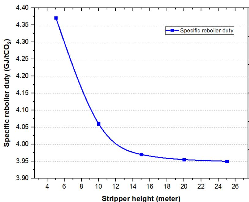
Figure 4.11. Relationship between the stripper column packing height and specific reboiler duty.
