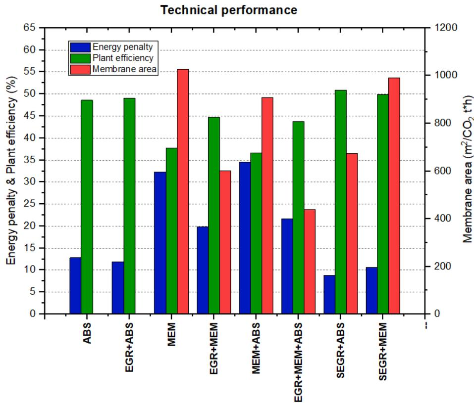
Figure 5.8. Comparison of energy penalty, plant efficiency, and required membrane area for each case.
