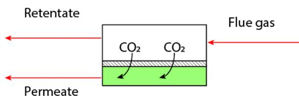
Figure 5.2. Basic flowsheet of membrane-based CO<sub>2</sub> separation process.
