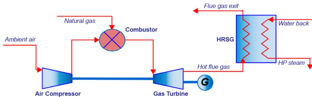
Figure 3.2. Turakurgan NGCC power plant’s simplified schematic figure.
