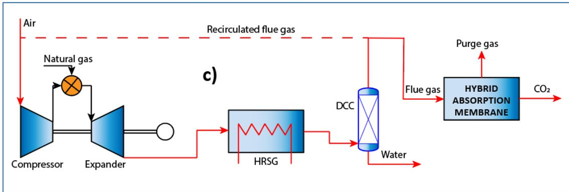
Figure 5.5. CO<sub>2</sub> capture by hybrid MEA absorption & membrane separation with EGR (case 5) and without EGR (case 6).
