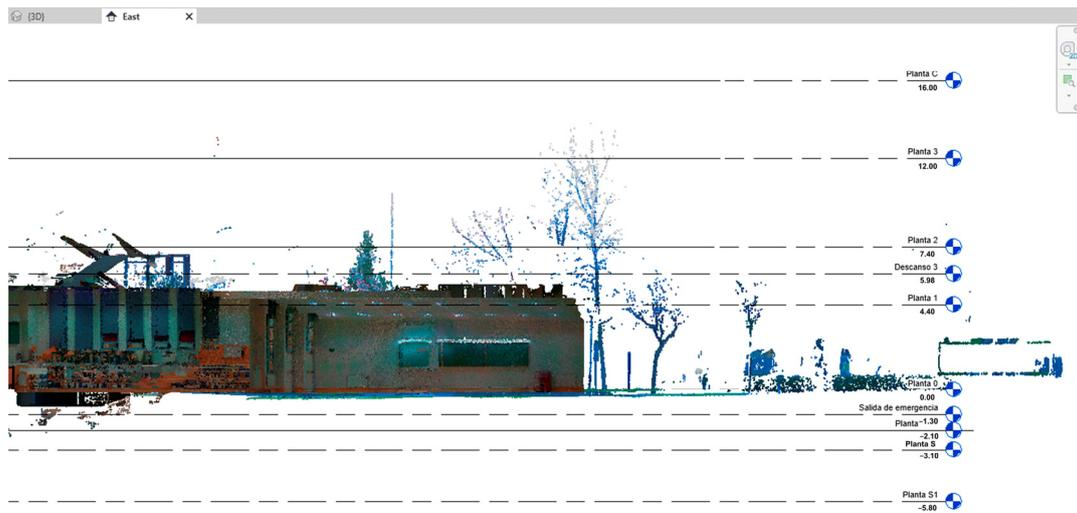
**Figure 13.** Process of readjustment of the model developed from existing plans, using as the template the point cloud resulting from laser scanning.
