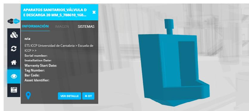
**Figure 21.** Selection and visualization of an individual asset in the men's restroom on the first floor of the Civil Engineering School within the 3D model. This feature allows users to view asset details, including their placement and condition within the facility.
