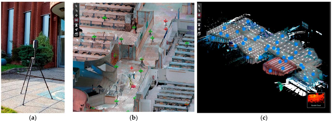
**Figure 9.** (a) Laser scanner Leica-geosystem BLK360. (b) Circular targets used in the laser scans visualized in linked point clouds. (c) General approach to the processing of the point cloud obtained from the first floor of the Civil Engineering School.
