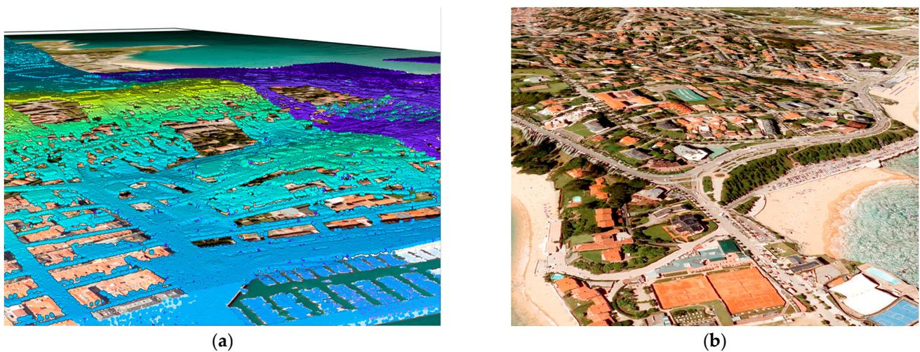
**Figure 7.** Terrain definition. (a) The point cloud from the 2012 LiDAR flight of the PNOA is displayed over an orthophoto of Santander. This combination allowed for a detailed visualization of the terrain and building features, enhancing the understanding of the geographical landscape and facilitating further analysis in GIS applications. (b) Textured digital terrain model (DTM) of Santander.
