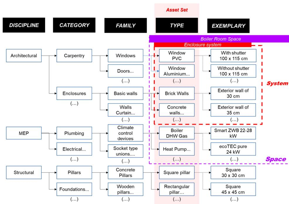
**Figure 5.** Hierarchical structure of the digital elements of the model.
