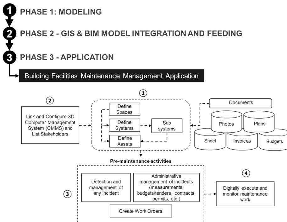
Figure 4. Procedure for managing the maintenance of the building’s facilities.
