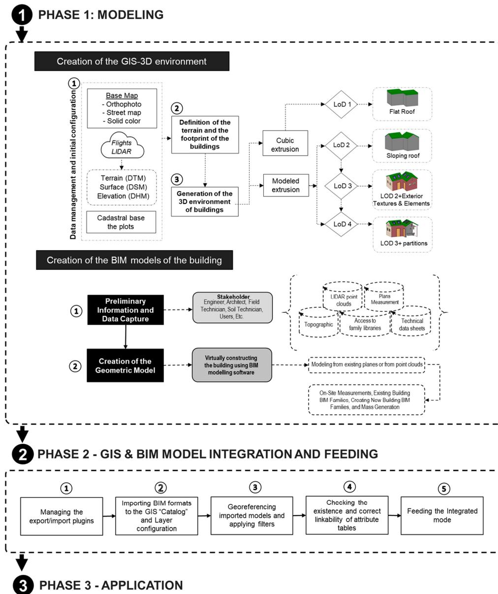
**Figure 3.** Schematic representation of the three phases of the proposed methodology for simulating 3D building facilities maintenance management.
