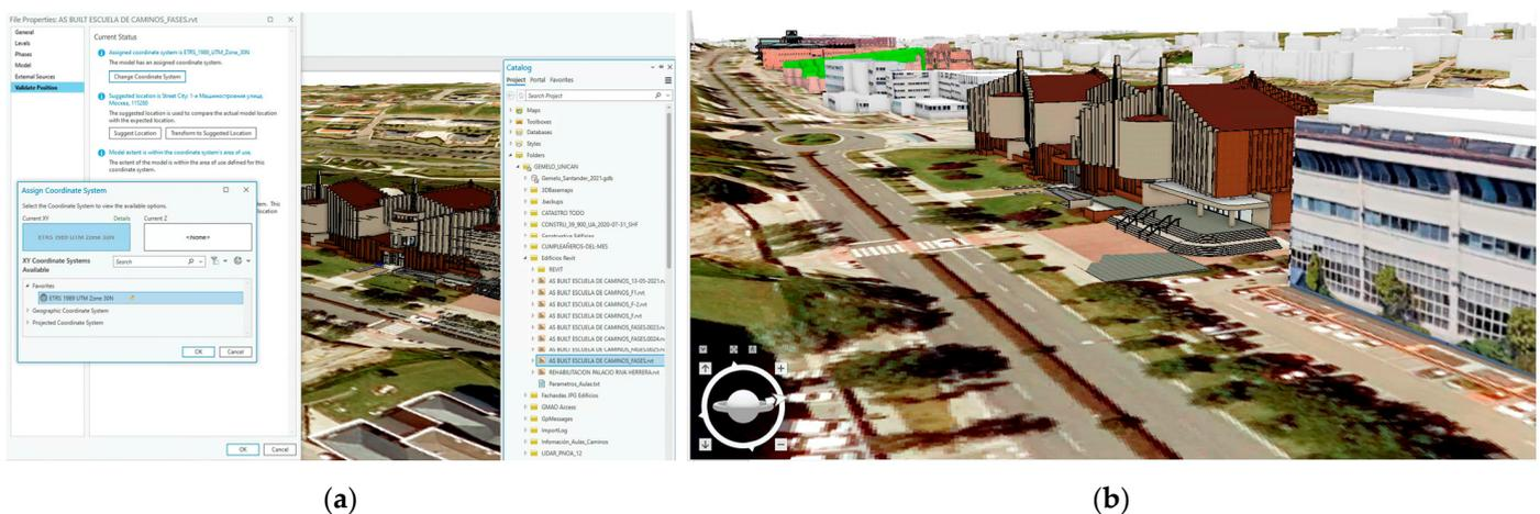
**Figure 14.** Model integration. (a) Georeferencing. (b) Integrated GIS and BIM model.
