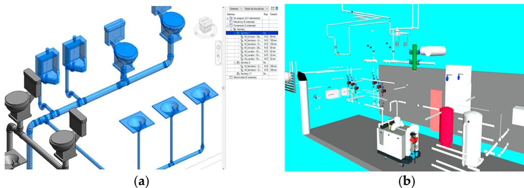
**Figure 18.** MEP (mechanical, electrical, and plumbing) modeling and system design for the Civil Engineering School. (a) Layout of sanitary fixtures in the men’s restroom located in the building’s hall, illustrating the arrangement and integration of various components. (b) Exploded view of the boiler system and its subsystems within the same building, offering a detailed perspective of the components and configurations to enhance understanding of the system’s functionality and design.
