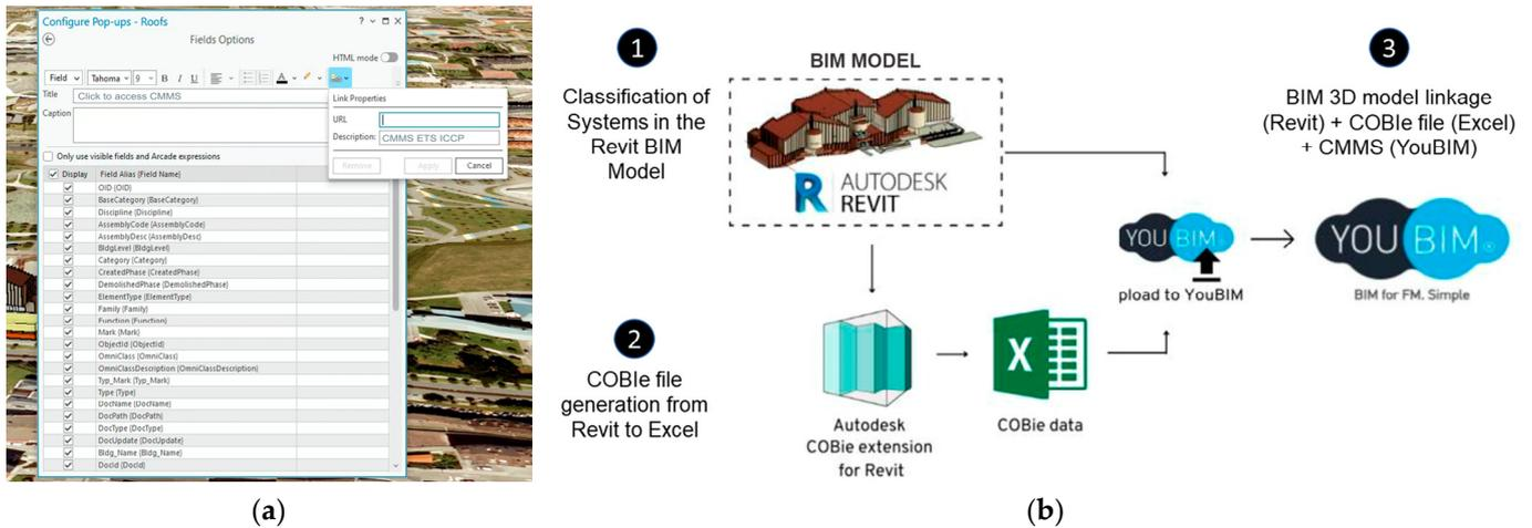
**Figure 17.** (a) Configuring the roof pop-up to add access to the CMMS. (b) Integration process of the BIM model with its data (COBie-Excel) to the YouBIM CMMS.
