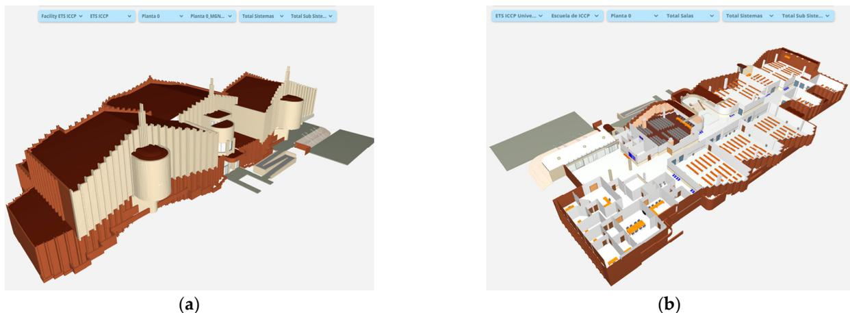
**Figure 19.** (a) The 3D navigation capabilities for the exterior of the Civil Engineering School model within the CMMS YouBIM environment. This feature enables users to interactively explore the building’s exterior, examining architectural features and surrounding elements. (b) A 3D visualization of assets within the CMMS YouBIM model. This feature offers an interactive representation of various assets, enabling users to examine their locations and interrelationships within the building.
