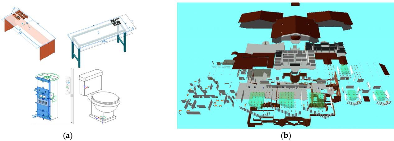
**Figure 15.** Preliminary BIM model input. (a) Preliminary feeding of the BIM model: examples of creation and edition of furniture and equipment families. (b) Equipment of the first floor of the building (authors’ elaboration with *eveBIM* software, version 4.2.4.585 [29]).
