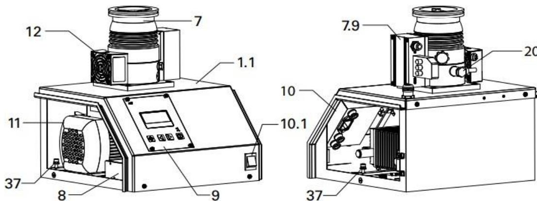
Fig 4: Components of the HiCube 80 ECO.
