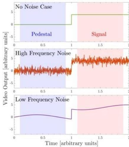
Fig 1.5: The top diagram shows a conventional CCD video output trace[7]. The down image shows a comparison of performing the CDS technique in a differential charge measurement in a case without noise, with high frequency noise components and a case with low frequency noise components[8].
