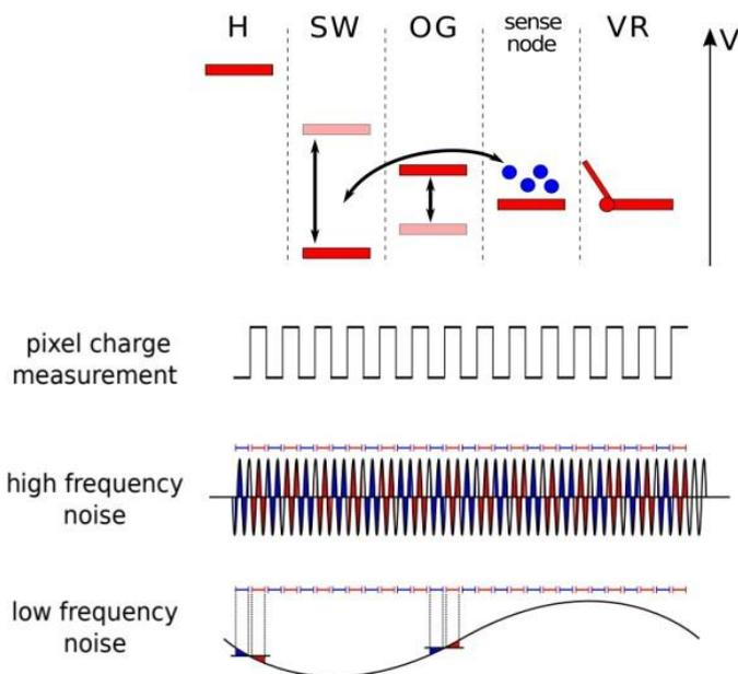
Fig 1.8: The pixel charge measurement of a skipper CCD. Here the low-frequency noise component is smaller. Figure from [6]
