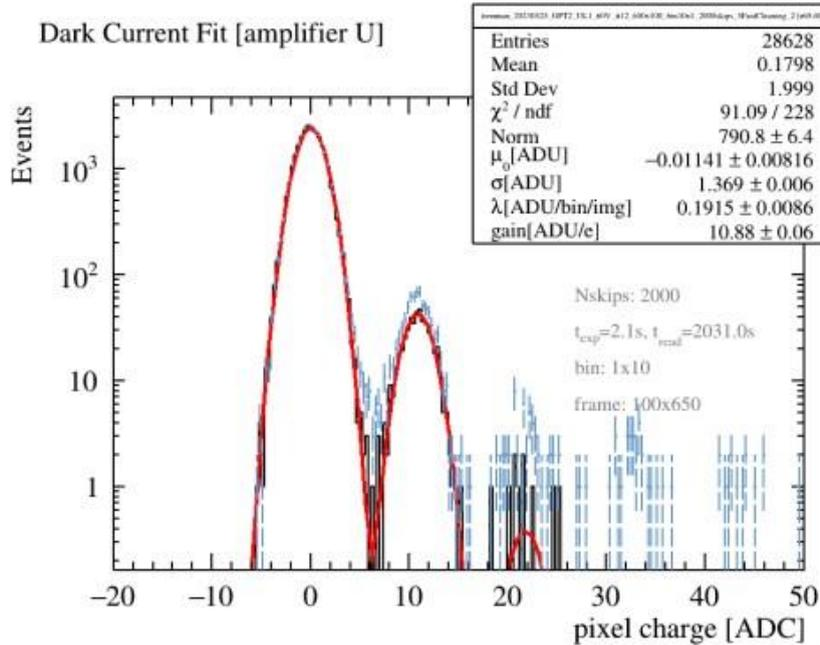
Figure 1.11: Dark current fit plot of an image taken with 2000 skips. The black histogram corresponds to the red histogram after the clustering and masking processes. The dark current rate  $\lambda$  (given in units of ADU per binning per image), the calibration constant  $k$  and the resolution (readout noise)  $\sigma$  are given by the dark current fit (red curve), i.e. the Gaussian-Poisson convoluted fit of the black histogram.
