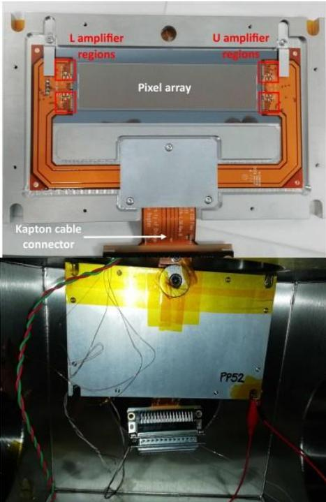
Fig 2: showing the inner and outer parts of the skipper CCD. Figure from[18].
