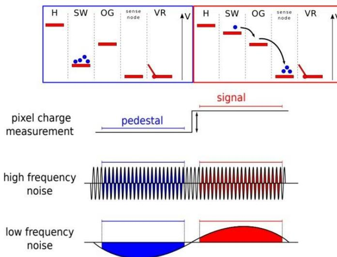
Fig 1.3: Showing pixel charge measurement of a conventional CCD. Figure from [6]
