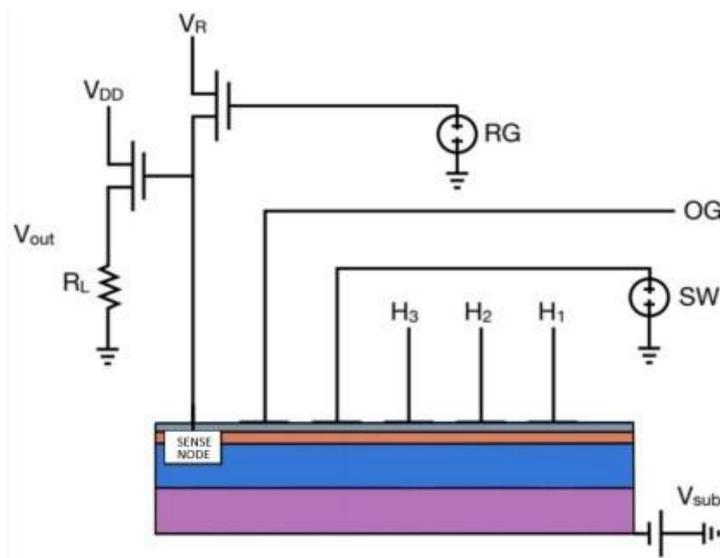
Figure 1.4: Circuit diagram of CCD readout. Picture from [7].
