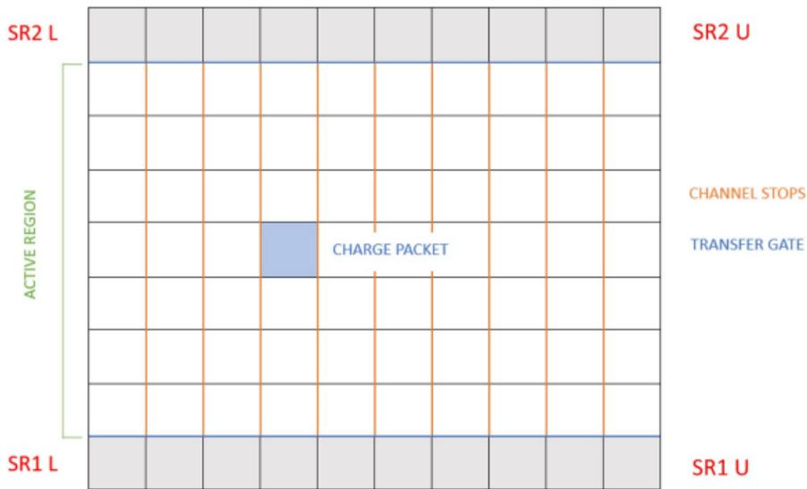
Figure 1.2: Diagram of the active region and serial registers (SR) of the CCD with labeled features.
