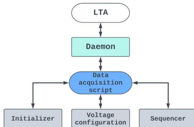
Fig 4.1: Block diagram of the main software components in the LTA.
