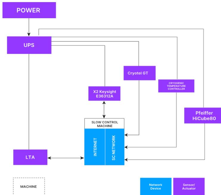
Fig 3.2 Schematics of the current configuration of the IFCA air-side electronics.
