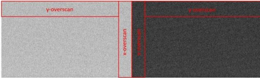
Figure 1.6: A non-skip image visualized with the “DS9” software. The left half side of the image has been taken with the left amplifier (L) while the right half side has been taken with the right amplifier (U). The x and y-overscans are labeled.
