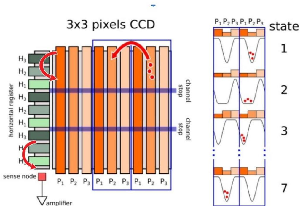
Fig1.1: Diagram of a CCD with a scientific readout system. At the right it can be seen the clocking sequence for transferring charge from one pixel to another. At the left is shown a put together picture of a CCD. Picture from [6].
