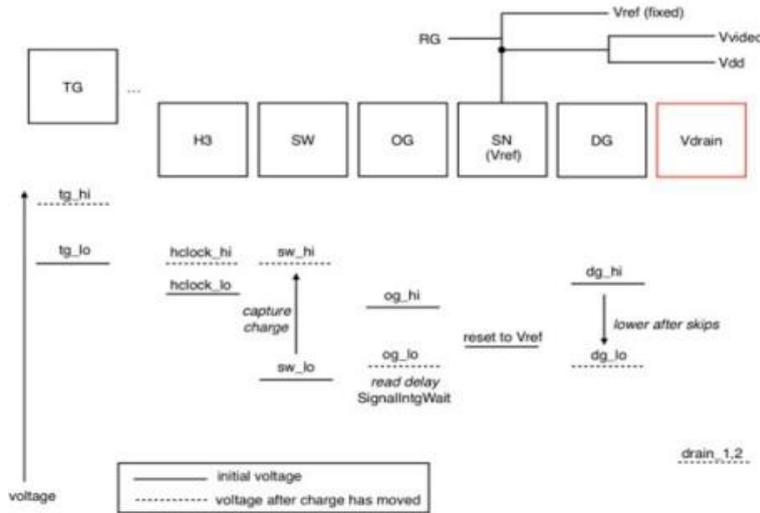
Figure 1.9: Diagram illustrating the structure of the output stage in a skipper CCD.
