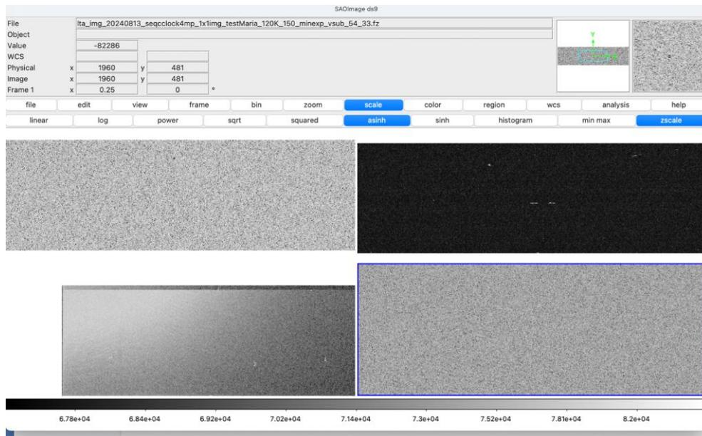
Fig 4.4: CCD images obtained by the setup at IFCA showing different tracks/ signatures for different ionizing particles in a CCD. A straight track (cosmic ray muon), large blob (alpha particle), “worm” (straggling electron) and small round clusters (low-energy X-ray, nuclear recoil, DM candidate)
