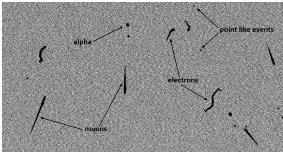
Figure 1.7: Diagram showing the image fraction visualized with “DS9” in which tracks produced by different types of particles are shown and labeled.
