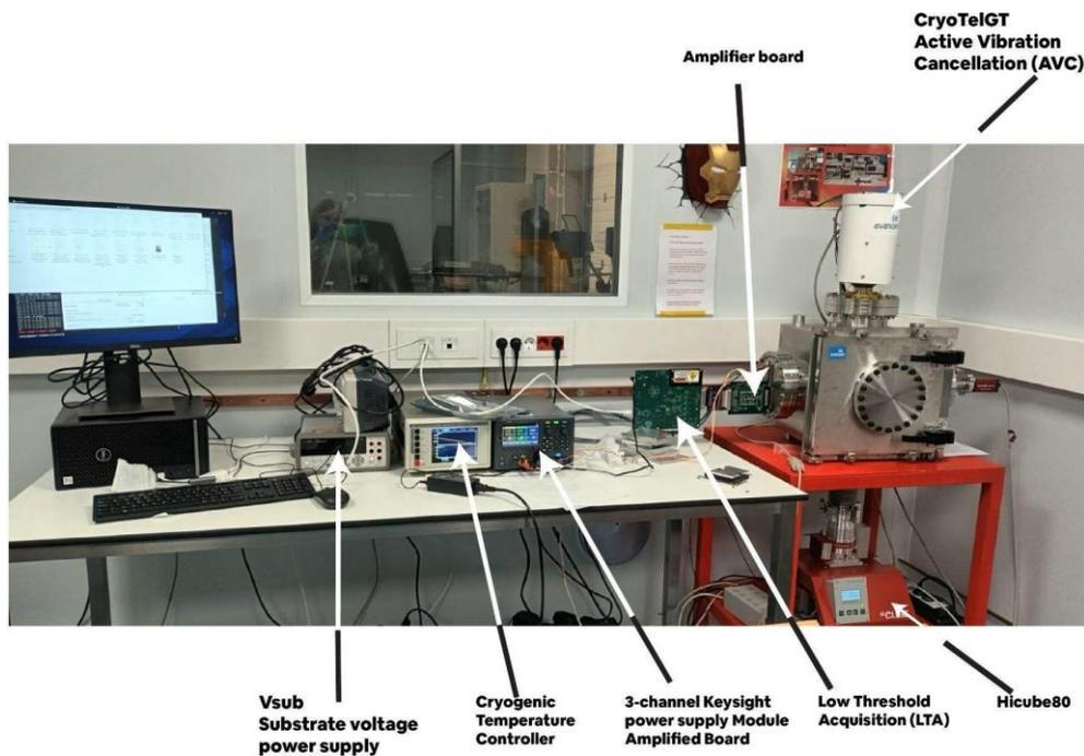
Figure 2.1: IRON MAN set-up for CCDs testing for DAMIC-M collaboration with labeled instrumentation.
