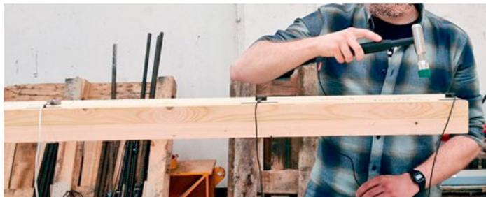
Fig. 3. Experimental modal analysis carried out in a duo-type glulam beam.
