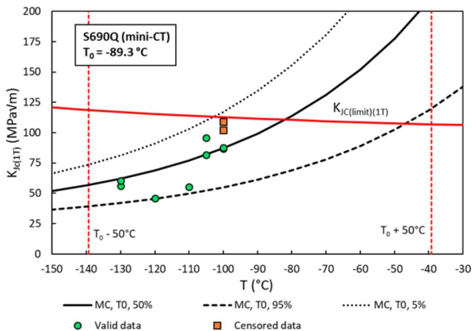
**Figure 6.** Steel S690 Master Curve obtained using mini-CT specimens, and comparison with the experimental results.
