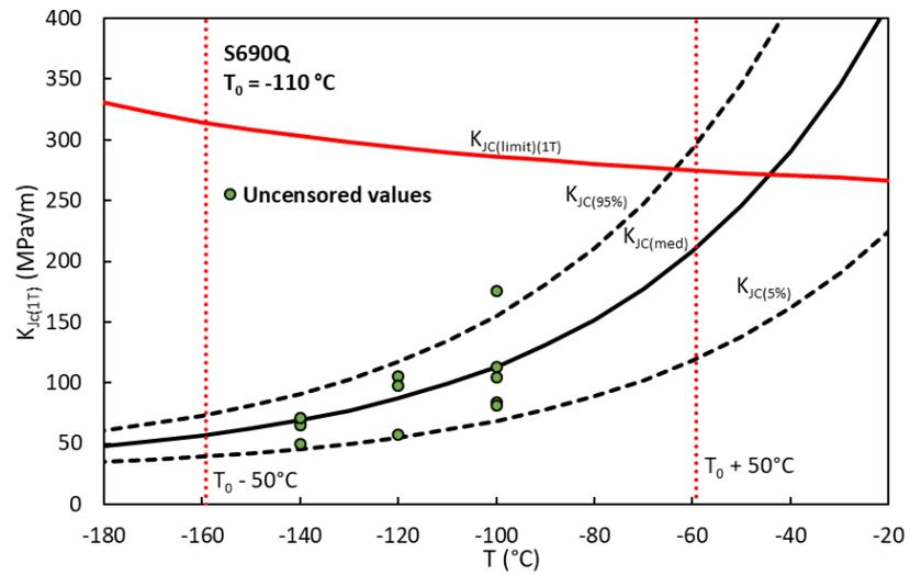
**Figure 3.** Experimental results of  $K_{Ic}$  (ASTM E1921) and resulting Master Curve. Steel 690Q, 0.6T SENB specimens.
