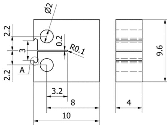
**Figure 1.** Geometry of mini-CT specimens. Dimensions in mm. Displacements measured on the front face.
