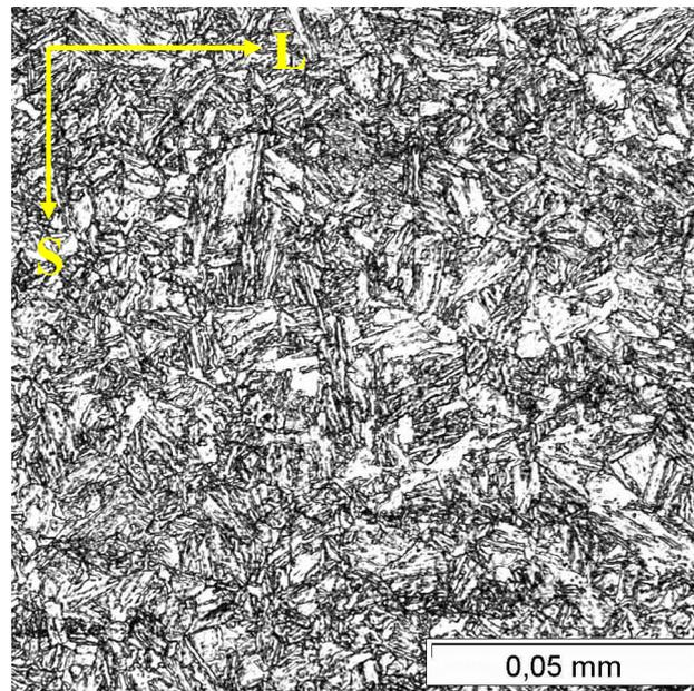
**Figure 2.** Microstructure of steel S690Q, showing L (rolling) and S (thickness) directions.
