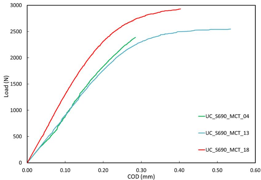
**Figure 5.** Examples of load-displacement curves obtained on mini-CT specimens.
