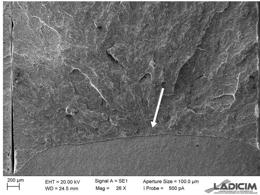
**Figure 7.** Example of fracture surface observed in mini-CT specimens S690\_04. The arrow indicates the location of the (single) initiation point.
