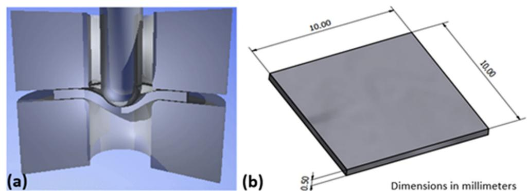
**Figure 1.** (a) Schematic of Small Punch test device; (b) SPT specimen geometry.
