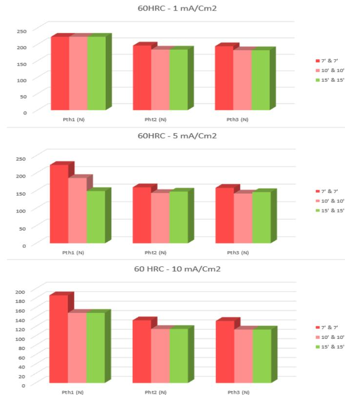
**Figure 9.** Threshold loads obtained under different step durations for the example case of 60 HRC steel in 1, 5 and 10 mA/cm<sup>2</sup> environments.
