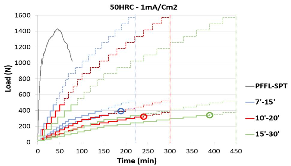
Figure 5. Step durations under study for 50 HRC steel in 1 mA/cm<sup>2</sup> environment.
