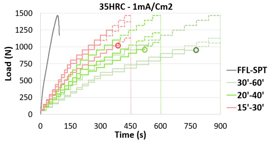
Figure 4. Step durations under study for 35 HRC steel in 1 mA/cm<sup>2</sup> environment.
