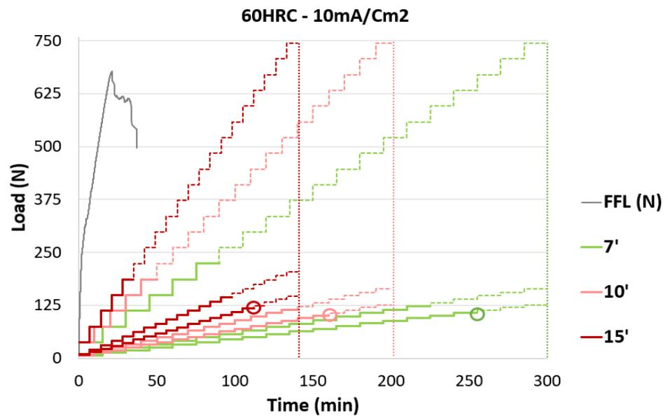
Figure 6. Step durations under study for 60 HRC steel in 10 mA/cm<sup>2</sup> environment.
