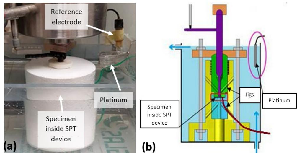
**Figure 3.** (a) Experimental setup to carry out the SPT tests while embrittling the sample; (b) schematic of its working principle.
