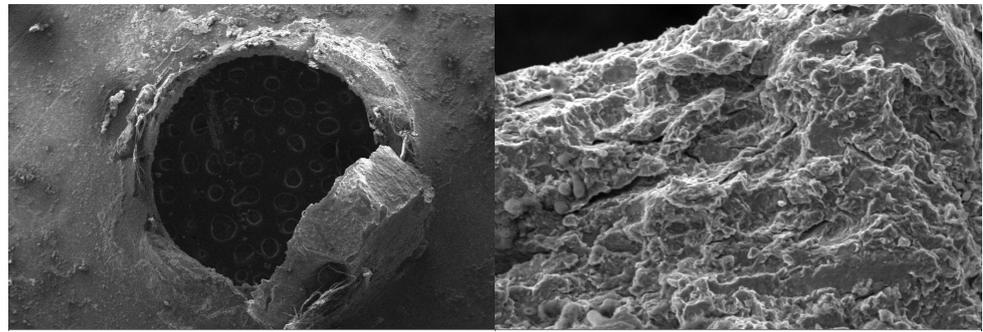
**Figure 10.** Example of SEM images corresponding to an SPT specimen of 35 HRC steel after being tested at  $10 \text{ mA/cm}^2$  for step times of 20 and 40 min (for steps 1–10 and 11–20). Macrography (**left**) and cross-section (**right**).
