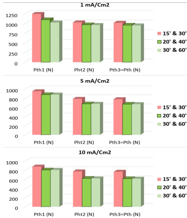
**Figure 7.** Threshold loads obtained under different step durations for the example case of 35 HRC steel in 1, 5 and 10 mA/cm<sup>2</sup> environments.
