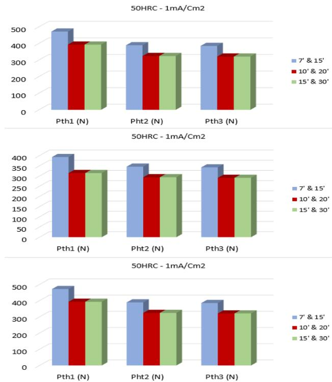
**Figure 8.** Threshold loads obtained under different step durations for the example case of 50 HRC steel in 1, 5 and 10 mA/cm<sup>2</sup> environments.
