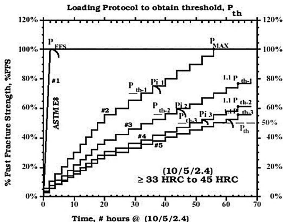
Figure 2. Schematic of the ASTM-F1624 methodology for a 33–44 HRC steel; extracted from [18].
