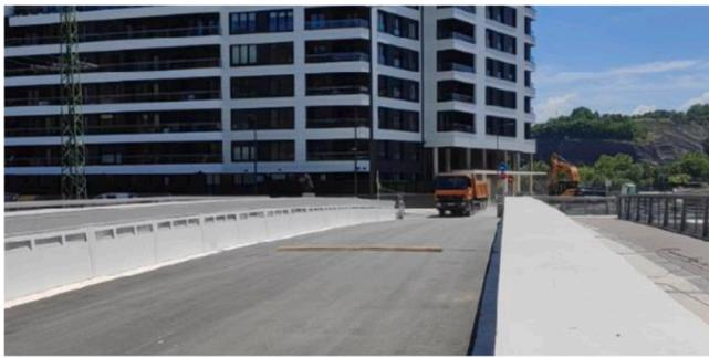
Fig. 21. Dynamic load test implementation.
