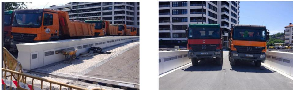
**Fig. 19.** Static test implementation. Configuration 2.
