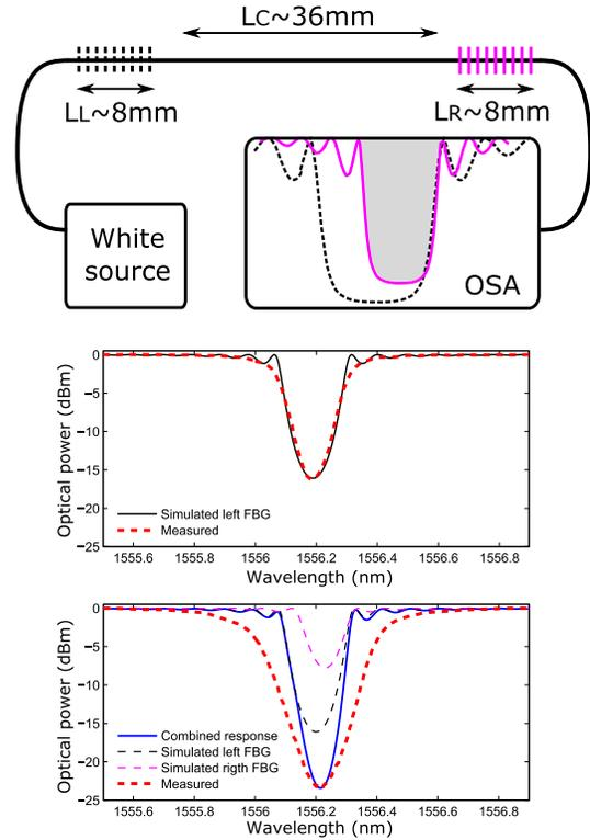
Fig. 2. Scheme of the DBR structure (top). Simulated left FBG parameters compared to its measured spectrum (middle). Simulated combined FBGs' response compared to their measured spectra (bottom).
