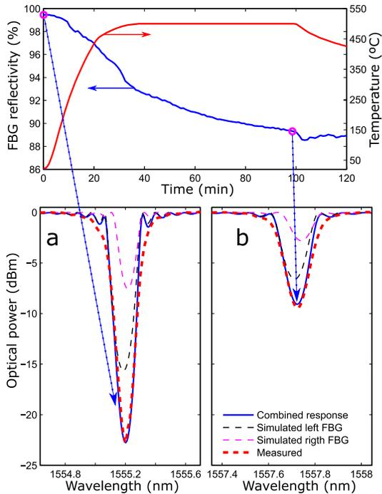
Fig. 3. Evolution of FBGs' combined response during the annealing (top). Simulated model of FBGs' response compared to their measured spectra before (a, aging  $\alpha_v = 0.98$ ) and after the annealing (b, aging  $\alpha_v = 0.54$ ).
