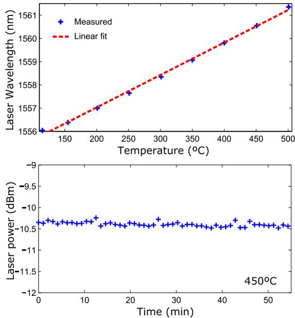
Fig. 5. Wavelength evolution of the annealed laser pumped at 980 nm (150 mA) during a temperature sweep (top). Power stability measured at  $T_w = 450^\circ\text{C}$  for 50 min (bottom).
