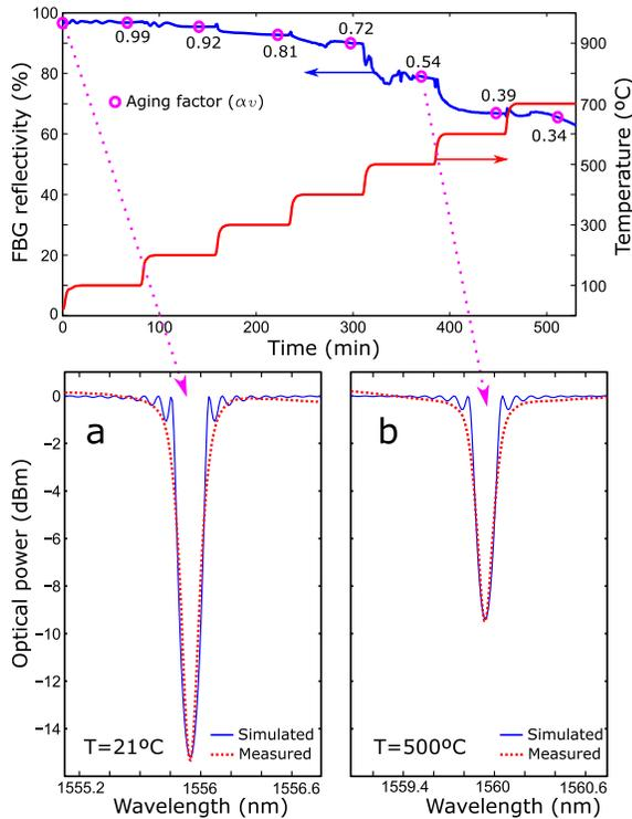
Fig. 1. Isochronal annealing of a 8mm length FBG written into Er-doped fiber. FBG reflectivity has been compared to the applied temperature sweep (top). Measured spectra (using an Agilent 86142A with a resolution of 60 pm) have been fitted to estimate their UV-induced index changes (bottom) at room temperature (a) and at  $T_a = 500^\circ\text{C}$  (b).
