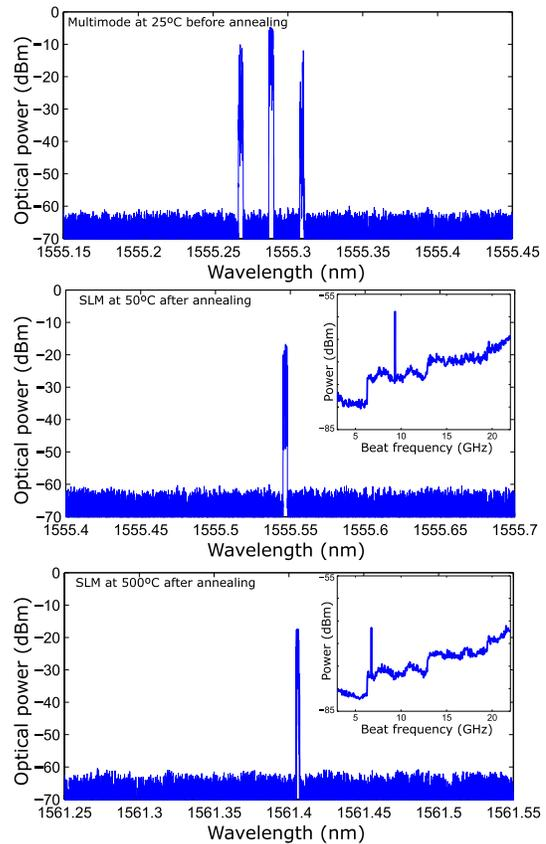
Fig. 4. Achieved longitudinal modes when pumped at 980 nm (150 mA) before the annealing (top), after the annealing (middle) and after the annealing but at high temperature (bottom). Captures with a heterodyne detection system to isolate the SLM regime at high and low temperatures.
