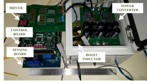
Fig. 14. Experimental prototype of the bridgeless sensorless converter and controller.
