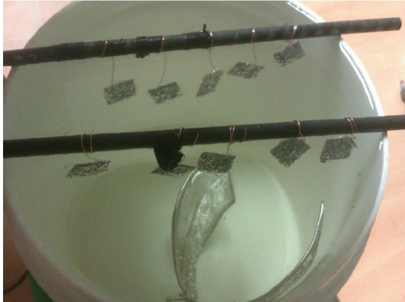
FIGURE 7. SPT PRE-EMBRITTLED SPECIMENS DURING ITS HYDROGEN ABSORPTION.
