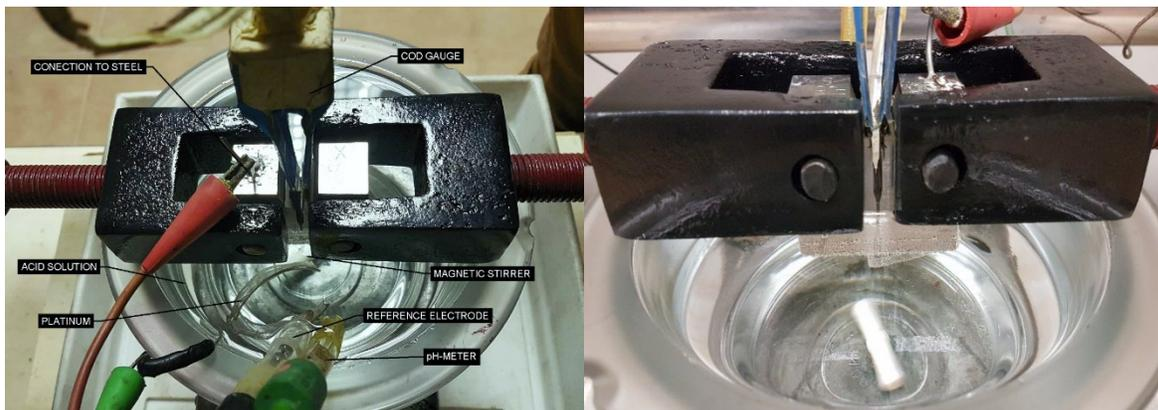
Fig. 5. Set up of the test under cathodic polarization.
