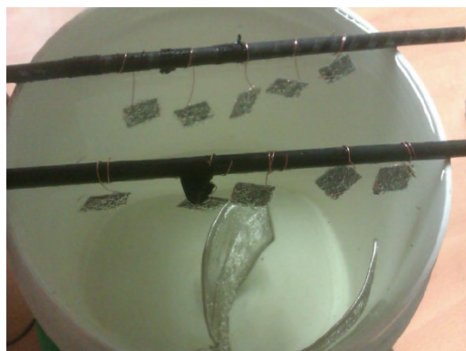
Figure 4. SPT specimens during its Hydrogen charge.
