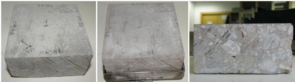
*Fig. 10. Concrete pavement sample before and after the tests*
