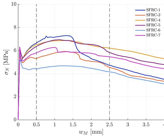
Fig. 10. Experimental three-point bending tests corresponding to the case study ( $\sigma_N-w_M$  relationship).
