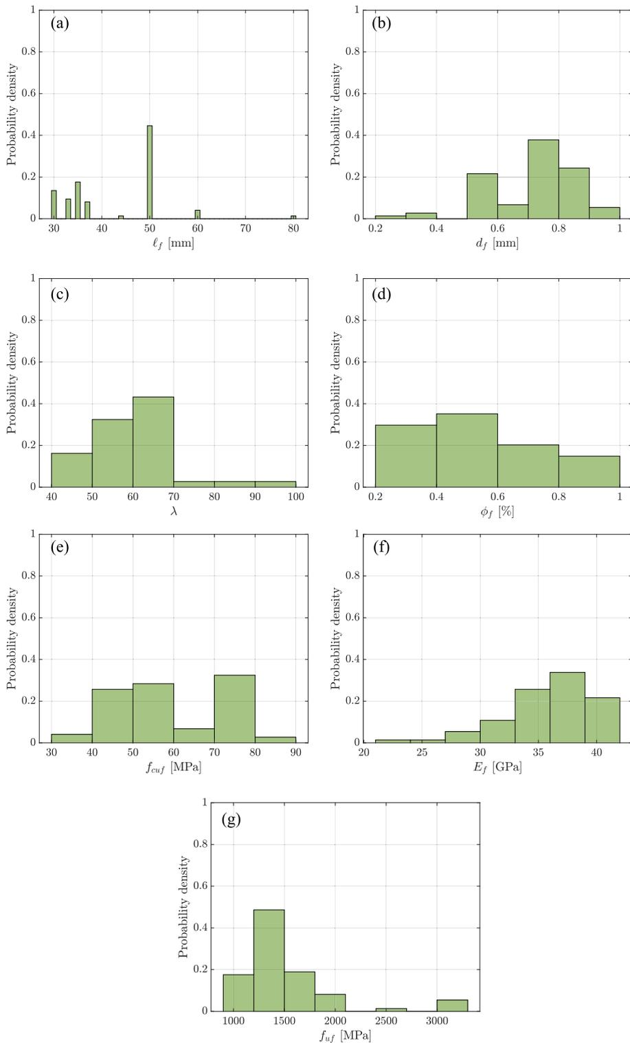
**Fig. 1.** Distribution of the data within the database: (a) non-dimensional fiber length ( $l_f^*$ ), (b) fiber diameter ( $d_f$ ), (c) aspect ratio ( $\lambda$ ), (d) volume fraction of fiber ( $\phi_f$ ), (e) compressive strength of SFRC ( $f_{cu,f}$ ), (f) elastic modulus of SFRC ( $E_{cf}$ ), (g) ultimate tensile strength of the steel fiber ( $f_{uf}$ ).
