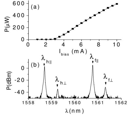
Fig. 1. (a) L-I curve and (b) spectrum of the free-running VCSEL ( $I_{bias}=5.5$  mA).
