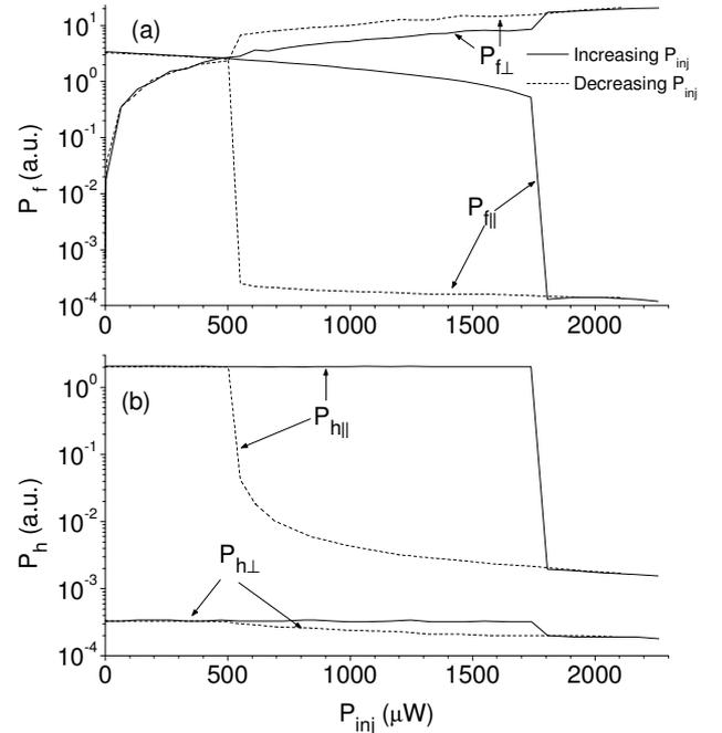
Fig. 6. Polarization-resolved I/O power characteristic for the output of the (a) fundamental and (b) high-order transverse mode.  $I_{bias} = 5.5$  mA,  $\Delta\nu = -10.75$  GHz.
