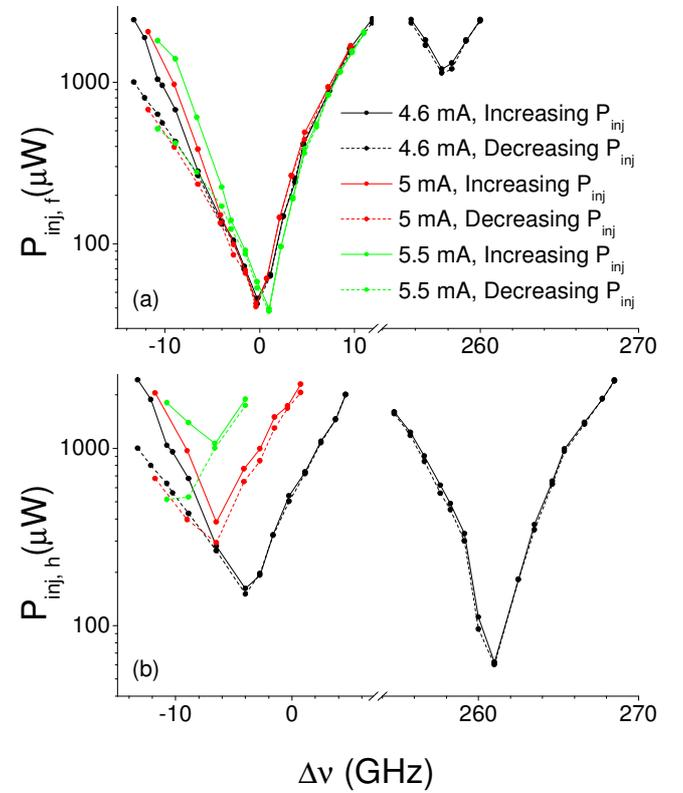
Fig. 4. (color online) Injected power required for suppressing the parallel polarized (a) fundamental and (b) high-order transverse mode versus the frequency detuning for three different levels of bias current. Results corresponding to increasing and decreasing the injected power are plotted with solid and dotted lines.
