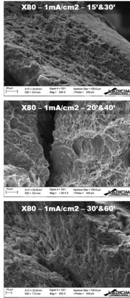
Fig. 11. Fracture surfaces of X80 steel obtained by applying the SPT step loading technique when tested in a cathodic polarization environment of 1 mA/cm<sup>2</sup>; images correspond to the sample tested under the final step protocol (the one that determines P<sub>th</sub>).
