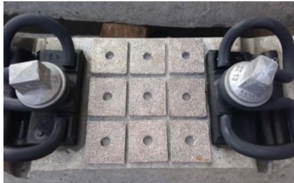
Figure 7. Layout of metal cushion samples behind the rail, to perform the electrical resistance test.
