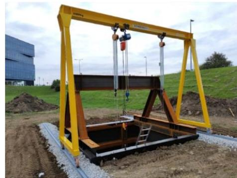
Figure 2. Testing container, loading frame and auxiliary crane.
