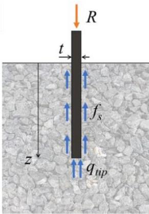
Figure 1. Plate penetration problem and calculation based on bearing capacity.
